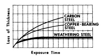
CORROSION RESISTANCE OF WEATHERING STEEL
