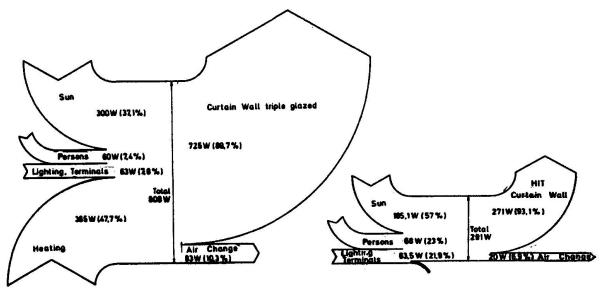
Mean power flux through curtain wall with triple glazing (left) and with HIT-window (right). Time: One week,  $\overline{I}_s = 98 \text{ W/m2}$
