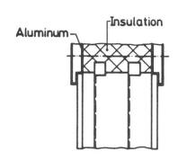
Fig 1 Schematic cross-section through HITwindow: frame (above), glazing (below)
