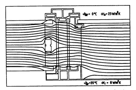
Temperature-distribution in HIT-frame and -glazing. Isotherms  $\Delta \vartheta = 1^{\circ}$ C. Left: glazing, middle: frame, right: curtain wall
