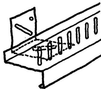
Fig. 13 Adjustable cladding rail
