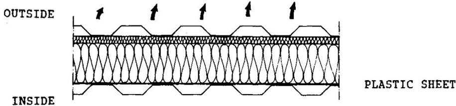
Higher inside air pressure: the plastic sheet is pulled towards the profiled sheet wall causing leakage
