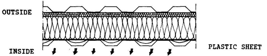
Lower inside air pressure: the plastic sheet is pressed against the ground plate and against the thermal insulation.
