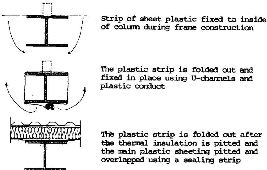
**Fig. 6** It can be difficult to place the plastic sheeting when steel columns are placed inside the facade. A strip of plastic sheet is therefore fitted directly after the completion of the frame and carefully fastened so as to avoid wind damage during construction. When the thermal insulation and the plastic vapour barrier are in place the strip is folded out to give a good overlap joint with the main plastic sheet.
