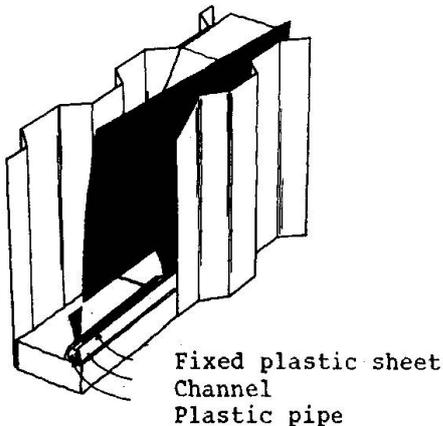
**Fig 3** If the plastic sheet is fixed in a channel with a plastic pipe, electric conduit for example, excellent air tightness is achieved.
