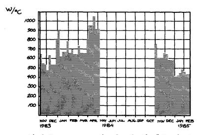
Fig 6 Energy consumption for the Ekerö Tennis Centre curing Nov. 1983-Feb. 1985. No recording during May 1984-Oct. 1984.
