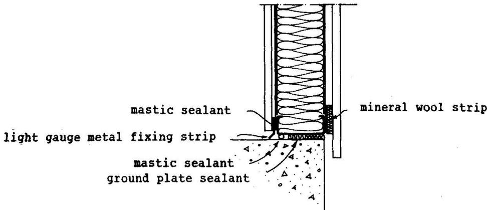
**Fig 4** An alternative method of achieving good air-tightness in the ground plate detail is to fasten the plastic sheet with a special light gauge metal fixing strip. A mastic sealant or sealing strip placed between the plate and the sheet will ensure air-tightness. The joint between the ground-plate and the concrete foundation slab must be well sealed; mineral wool with a joint sealant on the inside gives an acceptable result.
