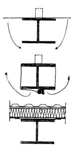
Strip of sheet plastic fixed to inside of column during frame construction
