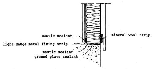
Fig 4 An alternative method of achieving good air-tightness in the ground plate detail is to fasten the plastic sheet with a special light gauge metal fixing strip. A mastic sealant or sealing strip placed between the plate and the sheet will ensure air-tightness. The joint between the ground-plate and the concrete foundation slab must be well sealed; mineral wool with a joint sealant on the inside gives an acceptable result.
