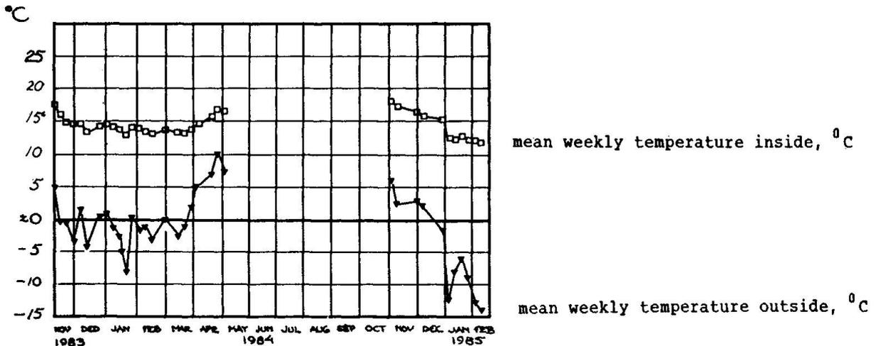
**Fig 7** Mean weekly temperature outside and inside respectively recorded at the Ekerö Tennis Centre during Nov. 1983 to Feb. 1985
