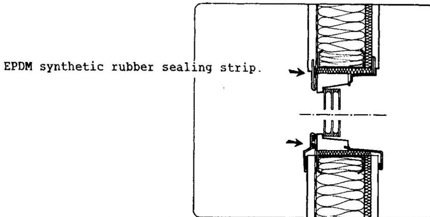
**Fig 7** Window detailing. The plastic sheet in the wall is drawn over the window frame and fastened with a special sealing strip. An EPDM synthetic rubber sealing strip between the plastic sheet and the window frame considerably reduces the risk for air-leakage.
