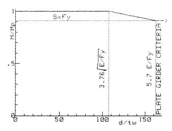
FIG. 3: LIMIT STATE WEB BUCKLING
