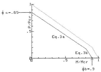
FIG. 8: INTERACTION CURVES FOR BEAM-COLUMNS
