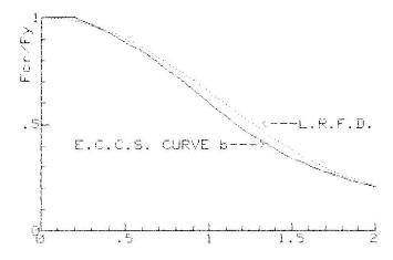
Fig.1: COMPARISON OF COLUMN CURVES
