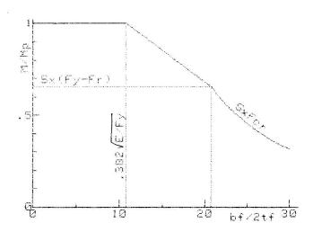
FIG. 2: LIMIT STATE FLANGE BUCKLING
