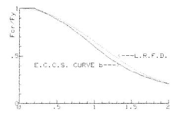
Fig.1: COMPARISON OF COLUMN CURVES
