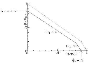
FIG. 8: INTERACTION CURVES FOR BEAM-COLUMNS
