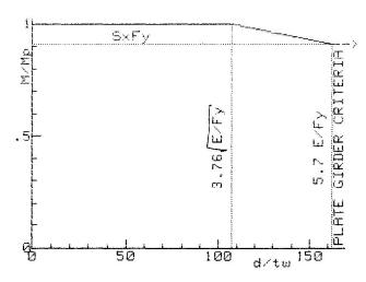
FIG. 3: LIMIT STATE WEB BUCKLING
