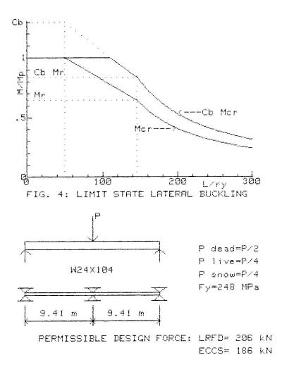
FIG. 5: BEAM DESIGN EXAMPLE
