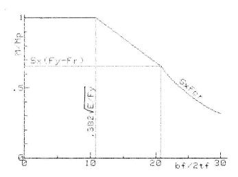
FIG. 2: LIMIT STATE FLANGE BUCKLING
