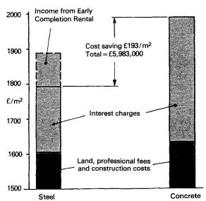
Fig. 9 Comparative building costs for 10 storey office block in London.
