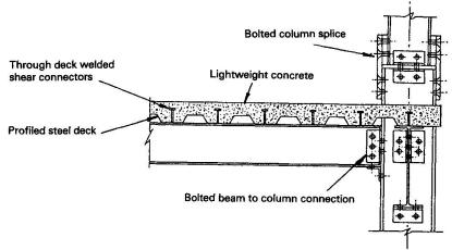
Fig. 2 Typical connection details.
