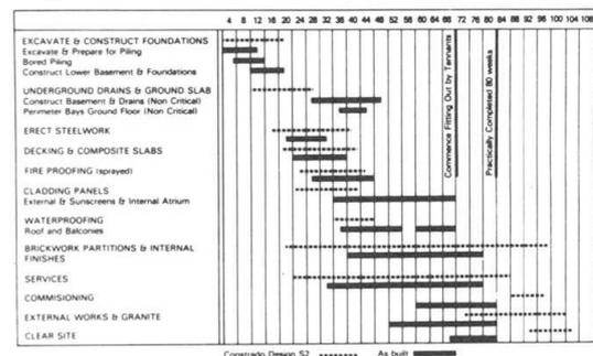
Equally striking is the progress schedule achieved on the nine storey Finsbury Avenue Development in the City of London. Using composite metal deck floors the project was completed four months ahead of the schedule for a comparably sized steel framed/metal deck building, included in the first edition of the Constrado cost study referred to earlier. (Fig. 6)
