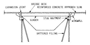
Fig. 3: Bridge with expansion joints
