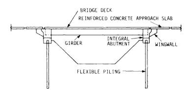
Fig. 2: Bridge with integral abutments
