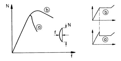
$\frac{\text{Fig. 1}}{\text{correlation-Diagram of an eccentrically loaded column and its}} \\ \\ \text{Load-Deformation-Diagram}$
