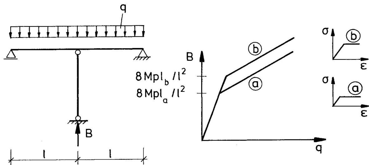
Fig. 2 Column load as a function of the plastic bending moment of the overlying girder
