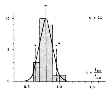
Fig.1 By Ingvarsson [1] and [2] observed ratio  $t = f_{CC}/f_{Ca}$  between strength in the finished structure  $(f_{CC})$  and the strength of corresponding standard cube specimens  $(f_{Ca})$ . n = number of observations. m = 0.80 (mean value). s = 0.10 (standard deviation). k = m - 1.65 s. k\* = m + 1.65 s.
