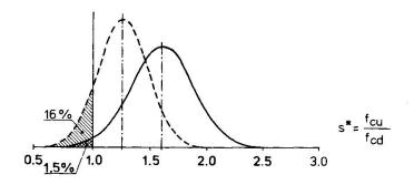
Fig.3 Structural safety  $S^* = f_{CU}/f_{Cd}$  when assuming Y = 1.1. The dashed curve shows the effect of delivering Grade K 30 concrete instead of specified Grade K 40 concrete.
