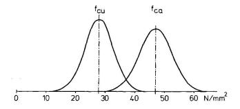
Fig.2 Compressive strength f<sub>Cu</sub> in a finished concrete structure of Swedish Grade K 40 concrete compared with the strength f<sub>Ca</sub> of the corresponding standard cube specimens.
