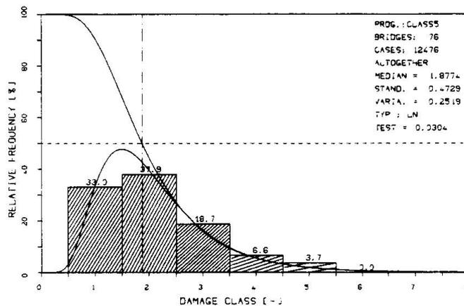
figure 4: Damage classes
