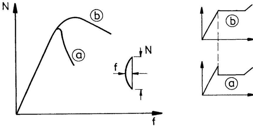
Fig. 1 Load-Deformation-Diagram of an eccentrically loaded column and its correlation with the Stress-Strain-Diagram
