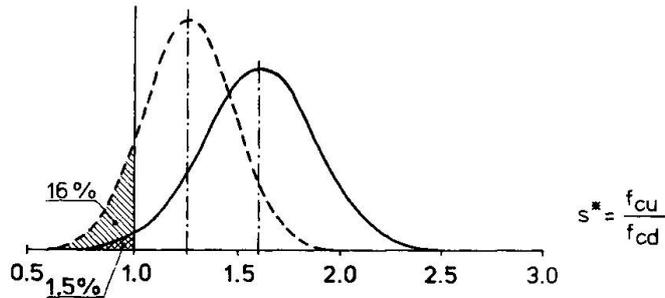
**Fig.3** Structural safety  $S^* = f_{cu}/f_{cd}$  when assuming  $\gamma = 1.1$ . The dashed curve shows the effect of delivering Grade K 30 concrete instead of specified Grade K 40 concrete.
