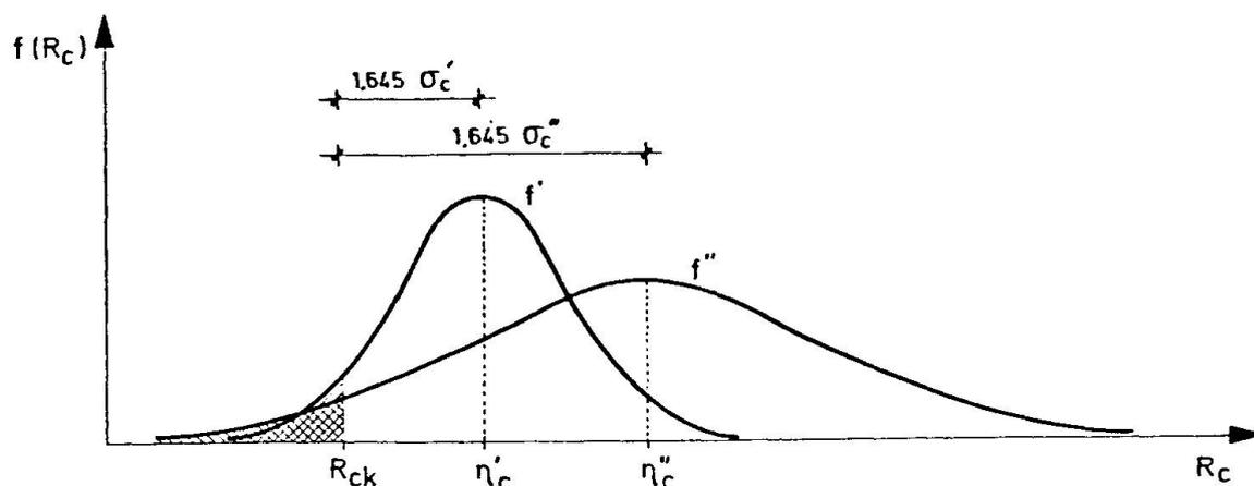
FIG. 1 Strength distributions of concrete
