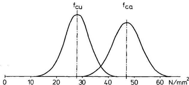
**Fig.2** Compressive strength  $f_{cu}$  in a finished concrete structure of Swedish Grade K 40 concrete compared with the strength  $f_{ca}$  of the corresponding standard cube specimens.
