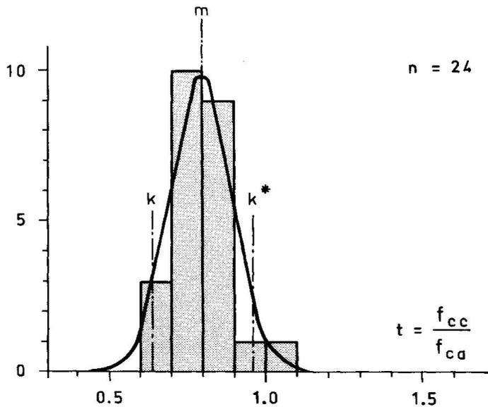
**Fig.1** By Ingvarsson [1] and [2] observed ratio  $t = f_{cc}/f_{ca}$  between strength in the finished structure ( $f_{cc}$ ) and the strength of corresponding standard cube specimens ( $f_{ca}$ ).  $n$  = number of observations.  $m = 0.80$  (mean value).  $s = 0.10$  (standard deviation).  $k = m - 1.65 s$ .  $k^* = m + 1.65 s$ .
