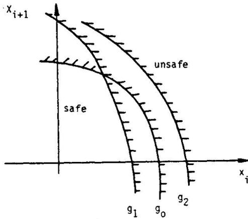
Figure 3: Failure domains for correct ( $g_0$ ) and false ( $g_i, i=1,2,\dots$ ) mechanical model
