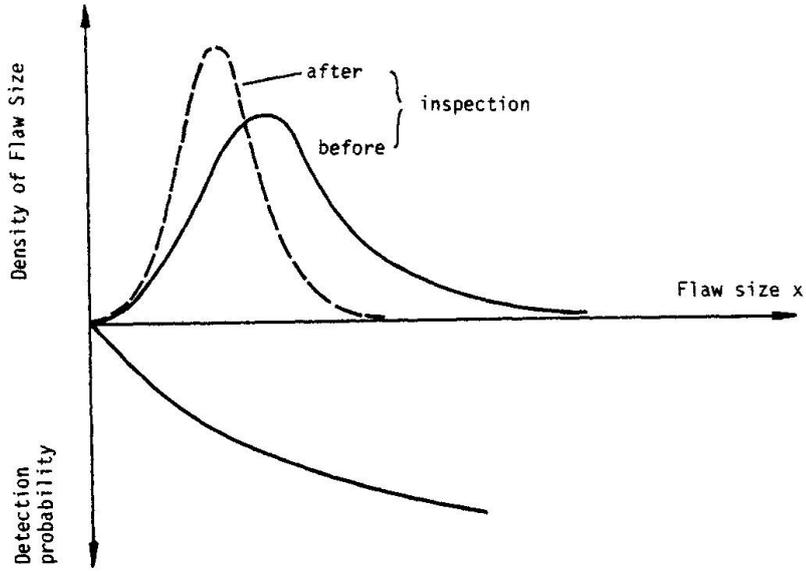
Figure 2: Flaw inspection and correction
