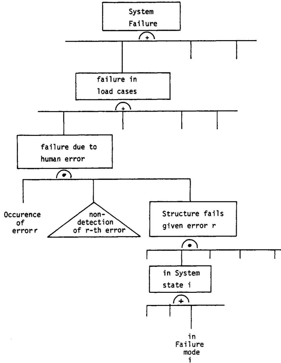
Figure 1: Fault (failure) tree of overall system
