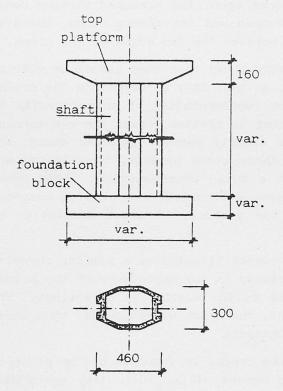
$\underline{\text{Fig. 1}}$  Schematic representation of the pier geometry.
