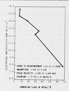
Fig.8: Relationship between electrical resistivity of concrete cored from field structures and metal loss.
