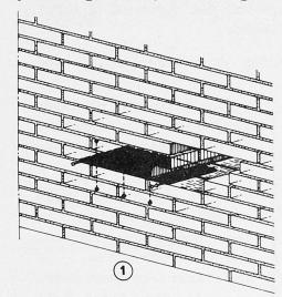
Fig. 6 Flat jack test.
