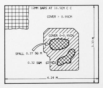
Fig.9: Distribution of concrete cover in spalled concrete
