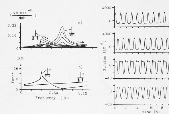
Fig. 5 Pier A: transfer functions (a) and exciting forces (b) for actual and "clamped" pier.
