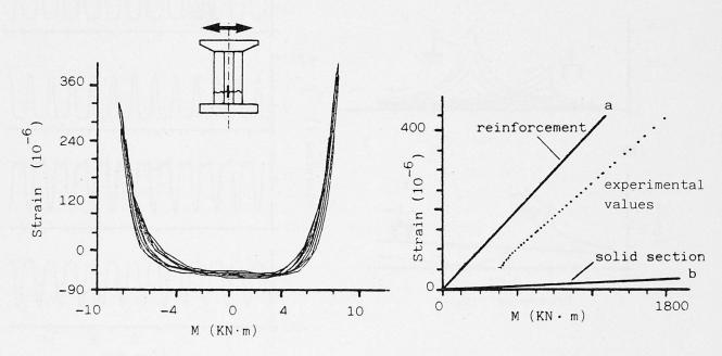
$\underline{\text{Fig. 9}}$  Pier B: strains measured versus overturning moment across a crack on the "neutral axis" of the shaft.
