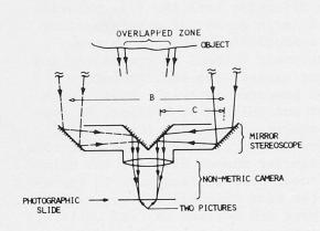
Fig.1: The mirror stereoscopic photographic arrangement
