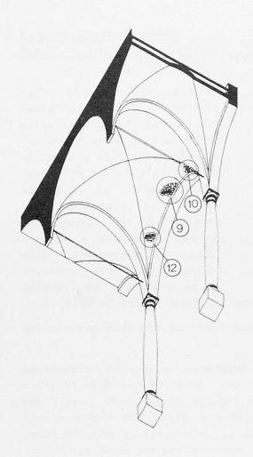
Fig. 7 Tests points on the cross vault.
