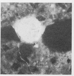
Fig. 6. Fluorescence. 160x. The same area as Fig. 5. Small cracks in the cement paste.
