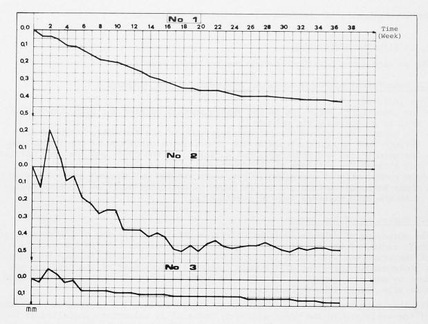
Fig.3 Variation of crack width with time
