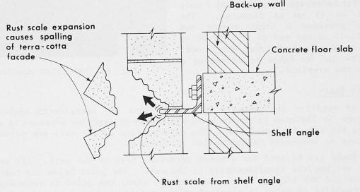
Fig. 3: Terra-cotta spalling caused by corrosion of shelf angle.
