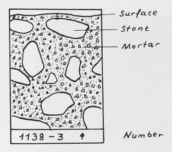
Fig. 4. Sketch of a thin section, 1:1.
