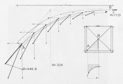
Fig. 9 Static solution adopted for cross vault.
