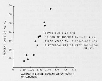
Fig.7: Relationship between Chloride content and metal loss.
