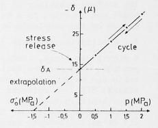
$\frac{\text{Fig. 10}}{\text{Tensile stress deduction}}$  from a pressure cycle p and corresponding displacements  $\delta$
