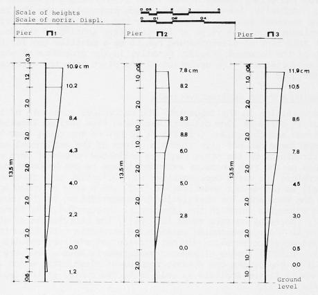
Fig.4 Horizontal displacements of the piers
