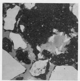
Fig. 7. Polarization. 65x. Badly mixed cement mortar with cement paste lumps and entrapped air. Big Ca(OH)<sub>2</sub>-crystals in the air pores.
