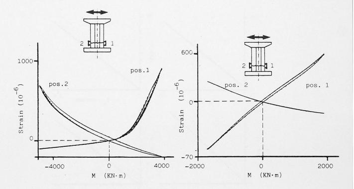
$\underline{\text{Fig. 7}}$  Pier B: strains measured across cracks versus overturning moment. The non symmetric behaviour of the crack openings is cleary shown.
