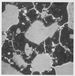
Fig. 8. Fluorescence. 65x. Dense cement paste with many micro cracks in a concrete containing silica dust.
