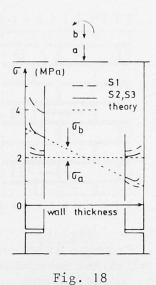
Stress measurement under two types of loading
