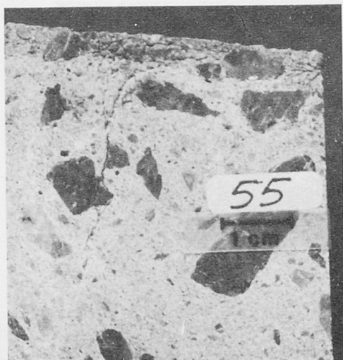
Fig. 1. Sawn cut of a concrete core with internal crack and low stone content.
