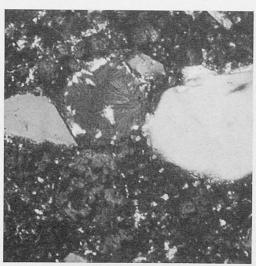
Fig. 5. Polarization. 160x. Air pore filled with Ca(OH)<sub>2</sub> and ettringite. Ca(OH)<sub>2</sub>-crystals in the cement paste.
