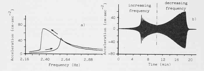
$\underline{\text{Fig. 3}}$  Acceleration values at top of the piers. a) Response curves for pier A; b) Time history for pier B. Tests with increasing and decreasing frequency.
