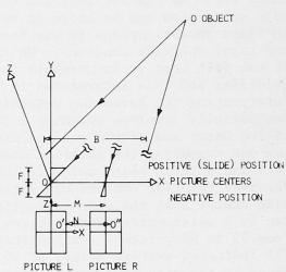
Fig.2: The geometry of the photogrammetric technique
