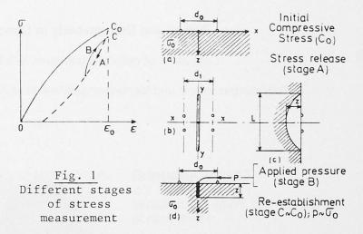
consists in a local elimination of stresses, followed by a controlled stress compensation (fig. 1). In practice, the displacement reference field is first determined; a slot is then cut in a plane normal to the desired direction of stress determination; finally, a very thin flat jack is introduced into the slot and used to restore the initial displacement field. The amount of cancelling pressure is an indication of the compressive stress in the direction normal to the slot.
