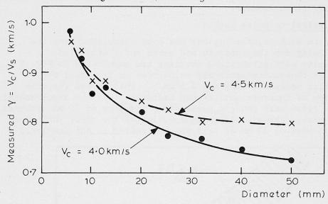
$\frac{\text{Fig. 6}}{\text{Effect of V}_{\text{C}}}$  and diameter for longitudinal bars
