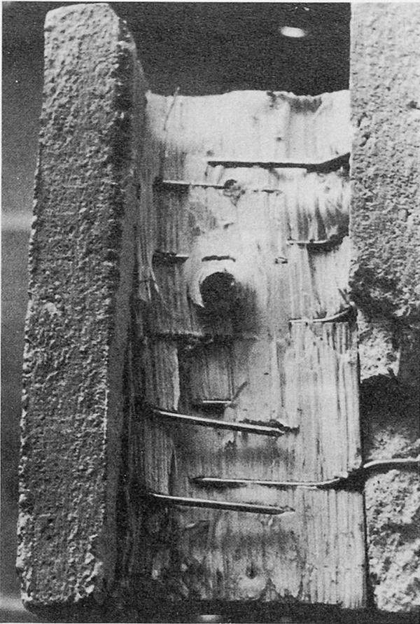
Fig. 9. Deformation of the nails after collapse
