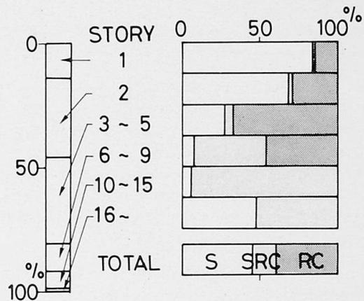
Fig.9 Usage of three types of structures (right) in different story buildings (left)
