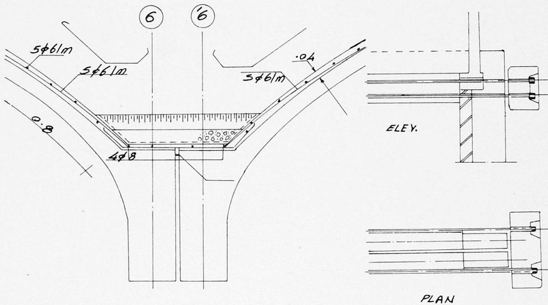
Fig.10 Repair Of Beams At Expansion Joints.
