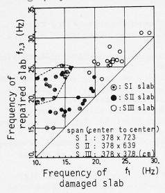
$\frac{\text{Fig.12}}{\text{of the slabs}} \text{ Increase of the Natural frequency}$
