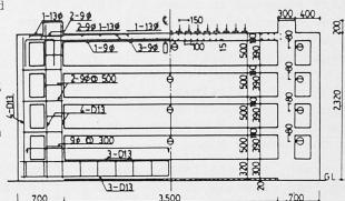
bar arrangement loading and measured points
