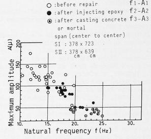
Fig.13 Relations between natural frequency and maximum amplitude
