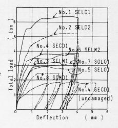
Fig.9 Load-deflection curves of the short-term loading tests
