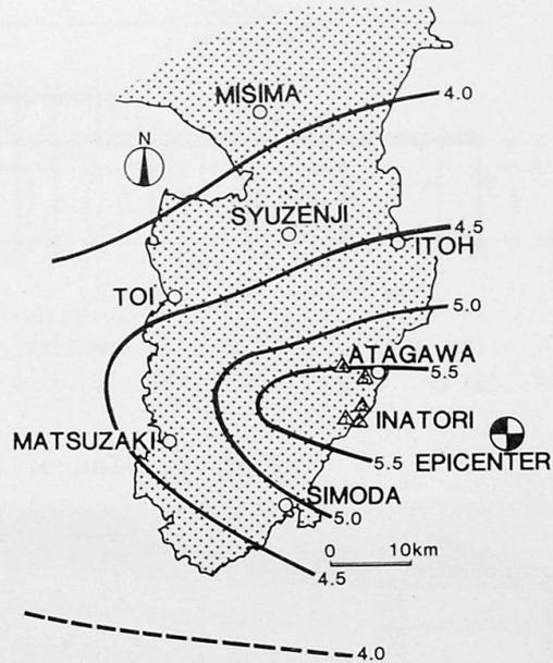
Fig. 2 Location of schools and seismic intensity([1])
