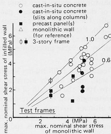
Fig. 7 Strengths of Infilled and Monolithic Walls
