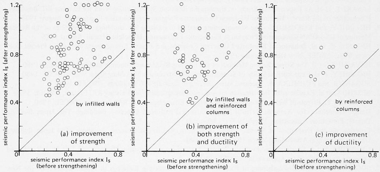
Fig. 16 Improvement of Seismic Resistance of Strengthened Buildings
