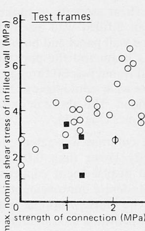
Fig. 10 Strengths of Infilled Wall and Connection
