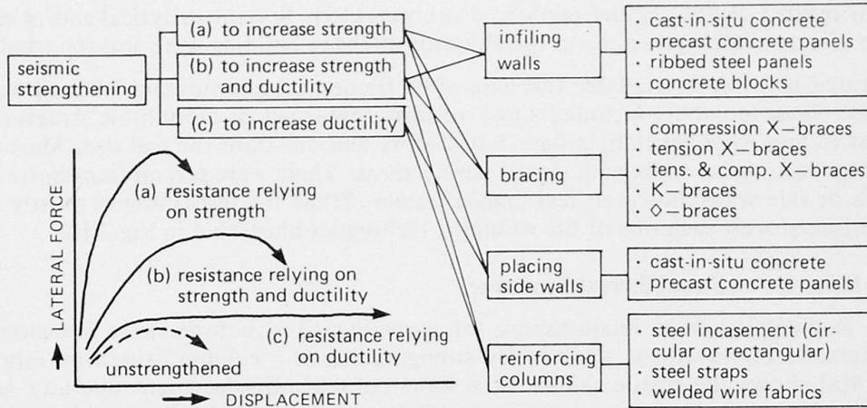
Fig. 1 Concepts of Seismic Strengthening and Strengthening Methods
