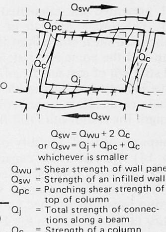
Fig. 11 Observed and Design Strengths of Infilled Wall
