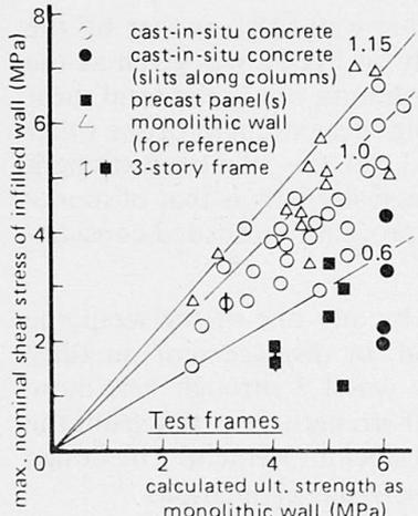
Fig. 9 Observed & Calculated Strengths of Wall
