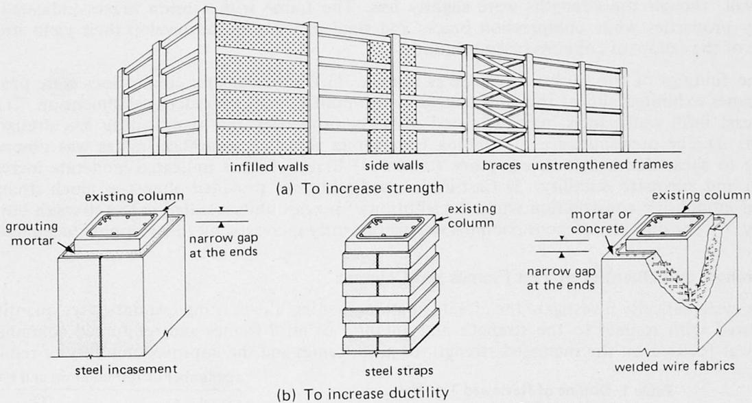
Fig. 2 Typical Construction Techniques for Seismic Strengthening
