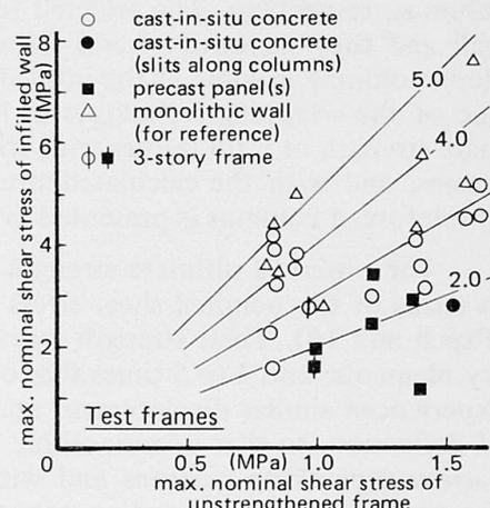
Fig. 8 Strengths of Wall and Unstrengthened Frame
