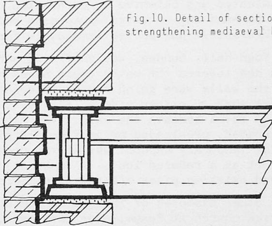
Fig.10. Detail of section: strengthening mediaeval building.
