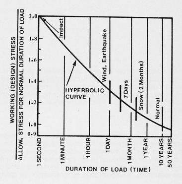
Fig. 1 Relationship Between Design Stress and Duration of Load
