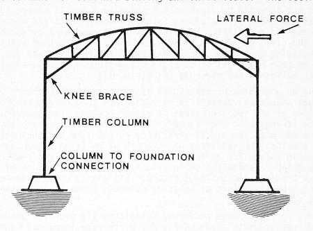
Fig. 3 Knee-Braced Truss Bent - A Structural System to Resist Lateral Forces
