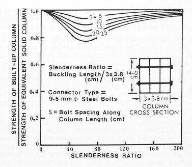
Fig. 2 Efficiency of Bolted Built-Up Timber
