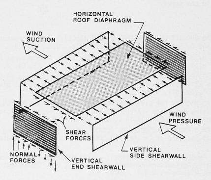
Fig. 4 Shearwall and Diaphragm Action in a Simple Building Subjected to Wind Load
