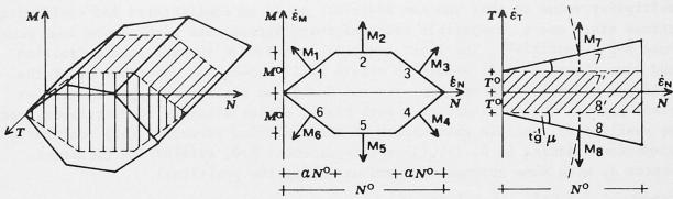
Fig.1 Elemental yield domains: axonometrie and sections.
