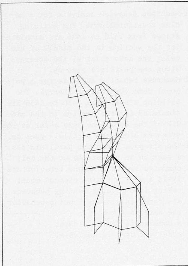
5-A finite element model of the dome structure for the analysis by no-tension behavior of the material.
