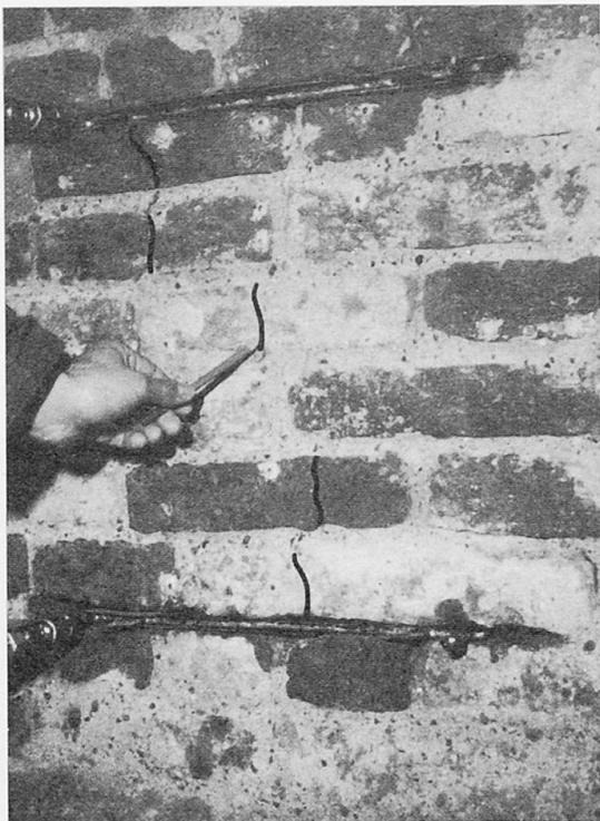
Fig. 12 Photo showing the appearance of first cracks.
