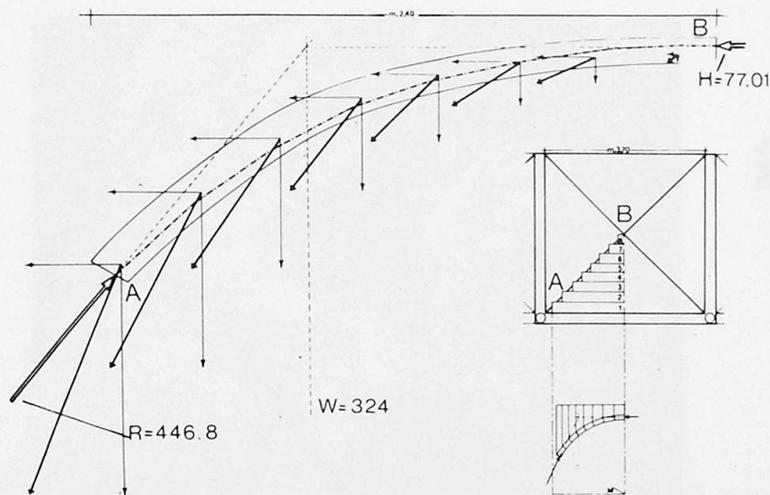
Fig. 9 Static solution adopted for cross vault.
