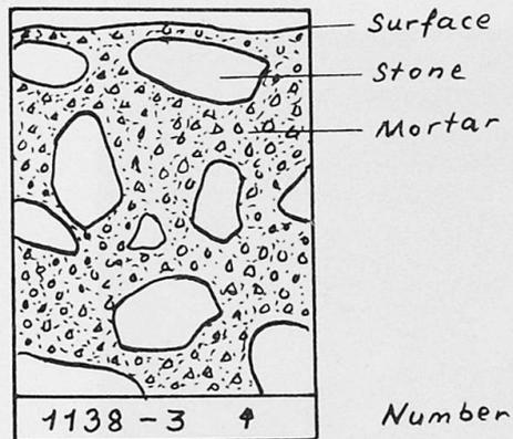
Fig. 4. Sketch of a thin section, 1:1.
