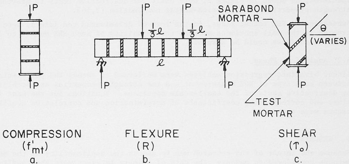
FIGURE 2 - SMALL-SCALE SPECIMENS
