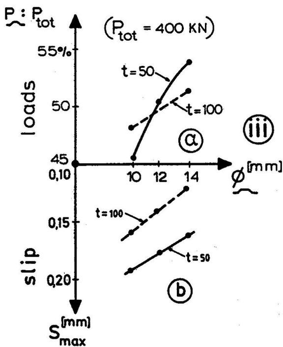
Fig. 40: Load transfer through R.C. jackets of damaged columns: i) Stress and deformations distribution along a jacket of length  $2a$ , ii) Computed results: load distribution and slips, as a function of loading, iii) The role of the diameter of the bend-down bars
