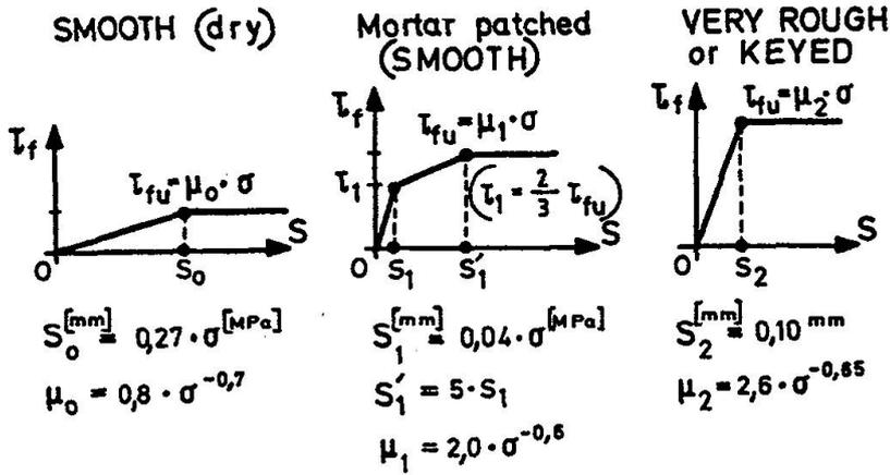
Fig. 6: Formalistic models for concrete-to-concrete friction, as a function of normal compressive stress "σ" (MPa) and relative displacement "s" (mm)
