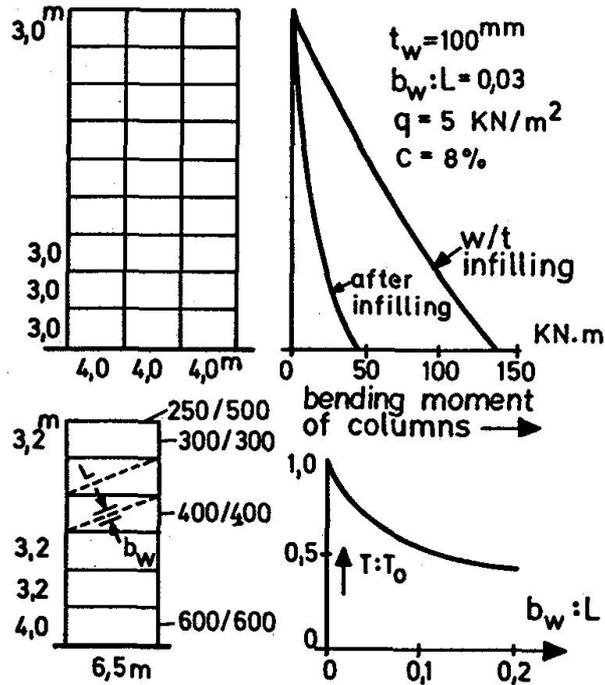
Fig. 54: Infill brick walls, drastically modify the structural behaviour of R.C. frames
