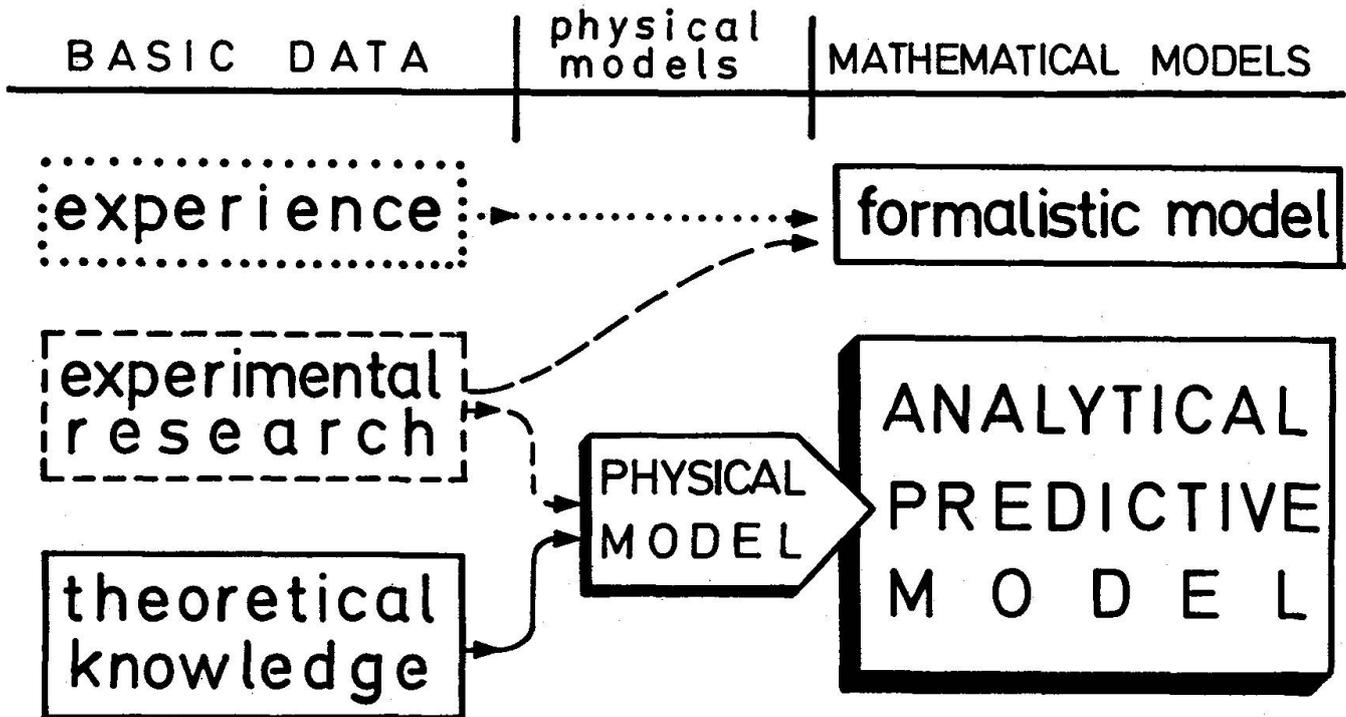
Fig. 2: A formalistic model is based on empirical data only and not on a physical model (i.e. on a rational knowledge about the structure and the function of the system described)
