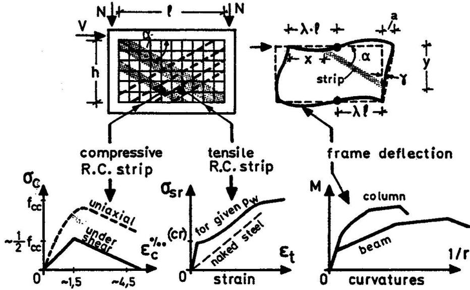
Fig. 43: Composite action of R.C. frame and R.C. infill wall, according to YAMADA et al., 1974.
