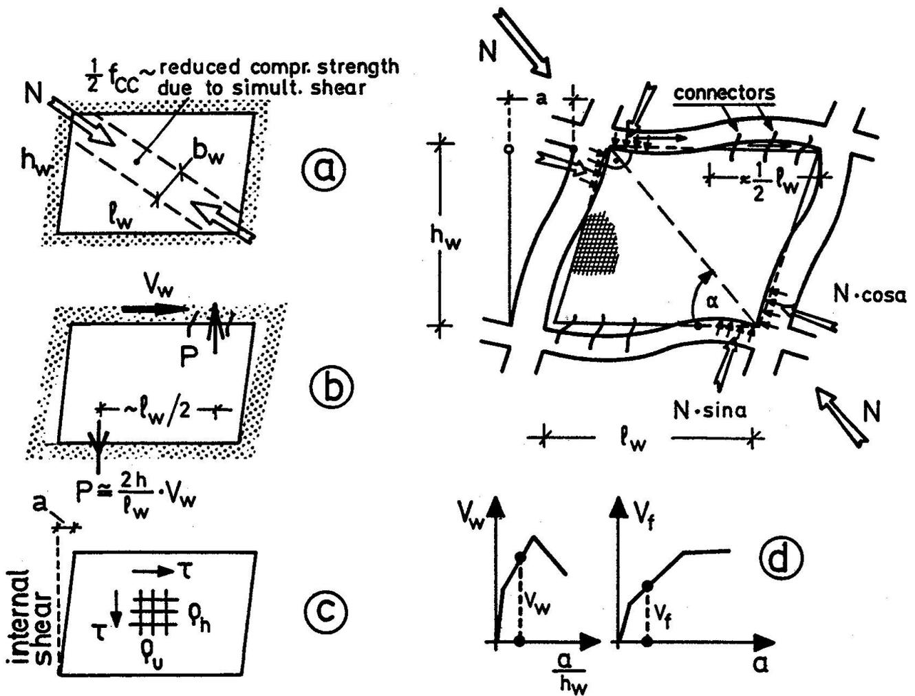
Fig. 44: Oversimplified model for dimensioning of infills
