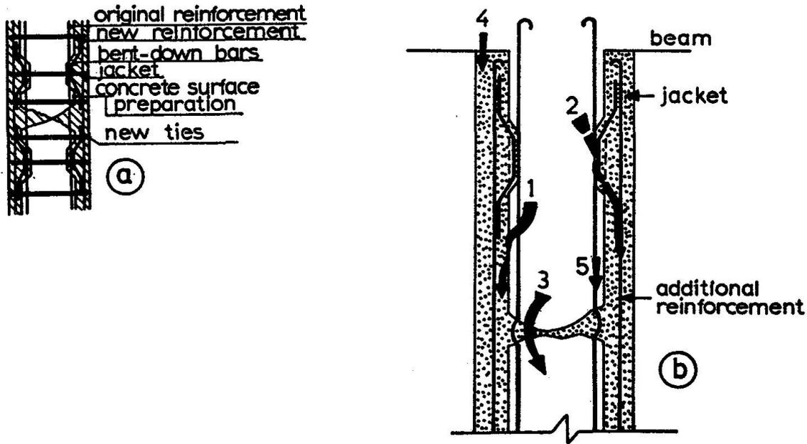
Fig. 38: a) Typical column repair by means of a concrete jacket
