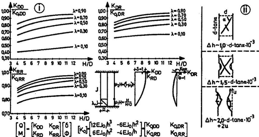
Fig. 50: i) Parametric calculation of stiffness indexes of a damaged R.C. column (Syrmakelis, Voyatzis, 1983) ii) Rough estimation of "settlement" of damaged columns
