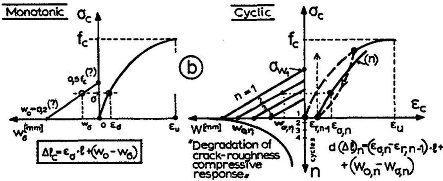
Fig. 3: Cyclic compression of pre-cracked concrete
