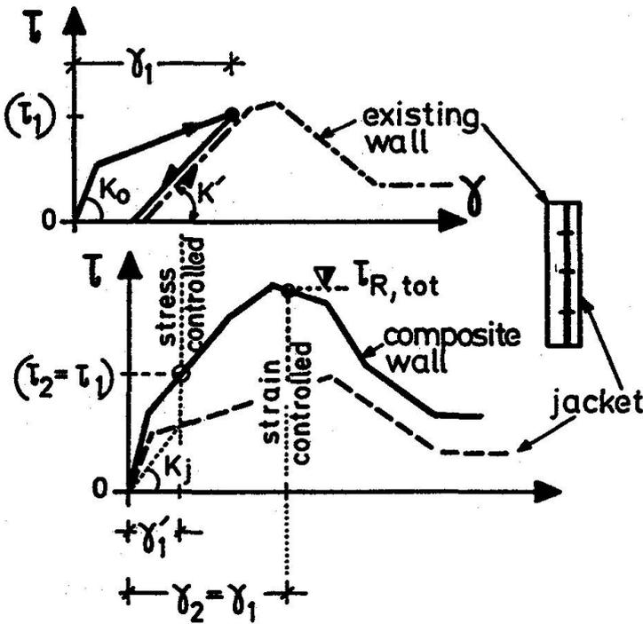
Fig. 46: Combination of existing R.C. wall (damaged at " $\tau_1$ "-shear level and unloaded) with a R.C. jacket; the composite wall is exposed to future stress  $\tau_2 = \tau_1$  or to future strain  $\gamma_2 = \gamma_1$
