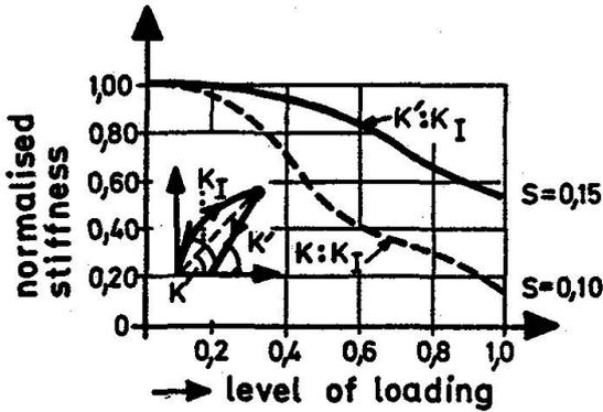
Fig. 31: Empirical values for residual stiffness after damage. A scattering equal to  $\pm s$  should be taken into account
