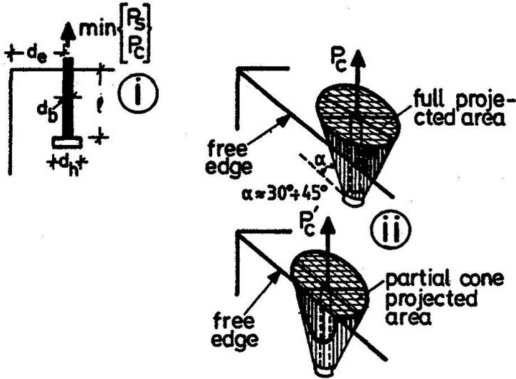
Fig. 45: i) Short anchors with anchorage head
