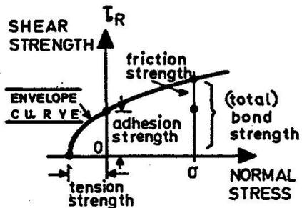
Fig. 4: Terminology regarding tension and shear strength
