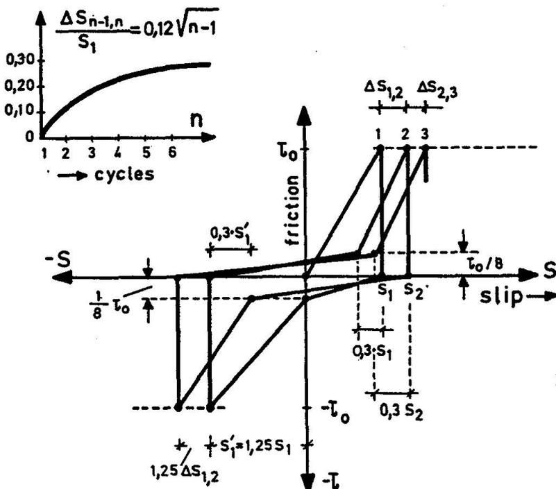
Fig. 8: A formalistic model for concrete-to-concrete friction under cyclic loading (based on Eleiott, 1974)
