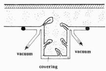
If the design of the beams is correct, i.e., made according to code specifications, stability problems should normally not arise; larger-thanaverage cracks, however, if they appear, should be closed in order to ensure the expected service life of the element.
