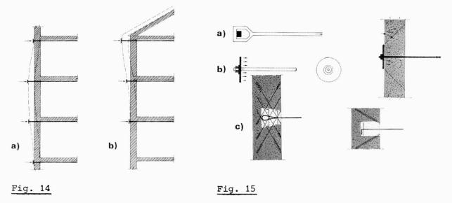
To avoid seing the anchor plates, the tie rods can be terminated into blocks, so metimes wedge-shaped as in fig. 15c, connected to the adjacent masonry by means of reinforced injections.
