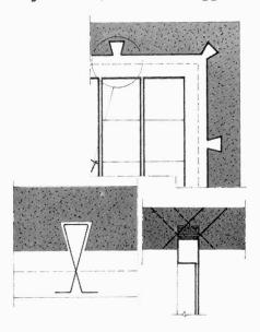
One way to realize the floor-to-wall connection can be that illustrated in fig. 18: V-shaped keys at the floor ends allowing also for the creation of a continuous concrete boundary element only slightly encased into the wall.
