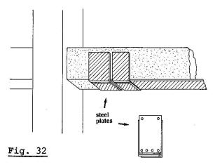
It consist in gluing steel plates on the element surface, using proper resin mixes. The adhesion between plates and concrete can be improved by treating the surface with acids. The main problem is the transmission of shear stresses within the concrete cover: to this purpose the plates are anchored into the body of the element by means of large con
