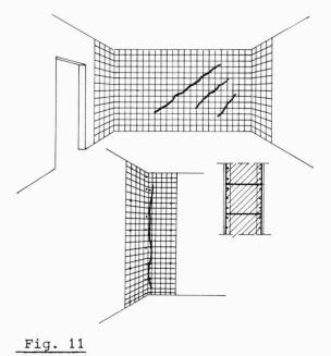
These coatings can also be used autonomously, without recourse to injections.
