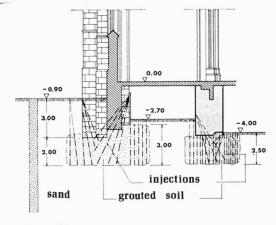
where first the cohesion is destroied by means of water jets, then it is restored with resin glues, thus obtaining strengths up to  $10 \text{ N/mm}^2$ .
