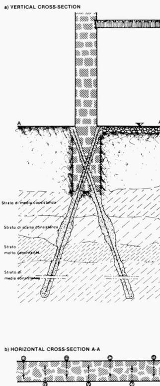
Due to their flexibility and ductility they are particularly suited for seismic areas, where they can be strongly reinforced.
