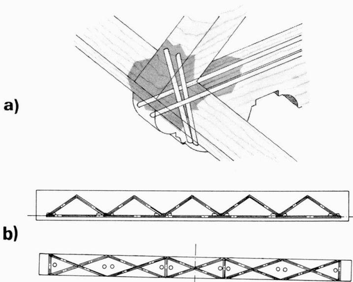
In some cases deteriorated parts of wood can be removed and epoxy mortars cast in situ to reintegrate them. This is frequently the case of the extremities of floor girders or trusses encased into niches of the walls and subject to humidity: the intervention can consist of the reconstitution of the degraded parts with epoxy resins, possibly with the addition of fiberglass, as shown in fig. 4.
