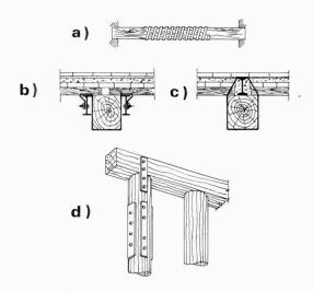
Connections between elements can be improved by attaching metal plates with bolts or nails (fig. 2d).
