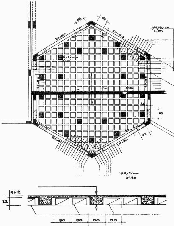
thickness having previously removed some of the tiles: small concrete blocks are thus created which act as keys improving the transmission of shear stresses (fig. 33). The extra thickness of the slab can be made variable with maximum at midspan, to save material and weight.
