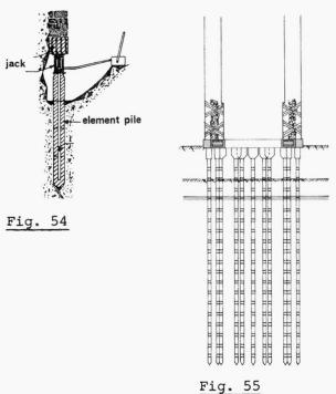
The jack driving the pile, this being progressively assembled in situ, counteracts on the structure itself.
