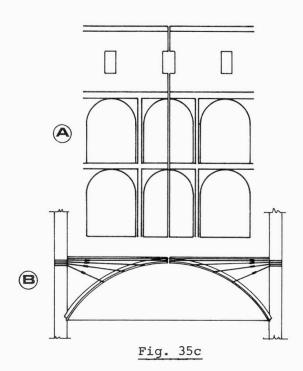
3.2 The differential settlements are obviously larger in case of nonhomogeneous subsoil. An example is provided by the Palazzo Ducale in Modena (fig. 35a), where a joint had to be inserted in correspondence to the variation of soil type (35b). In this case differential settlements were also due to subsidence phenomena. It is visible in the figure the cut crossing a vault (35c).
