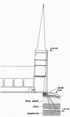
means, the one of the Lubeck Cathedral must be cited (fig. 58): after the strength ening of the masonry edge, a local pressure has been applied, counteracting on ad hoc piles.
