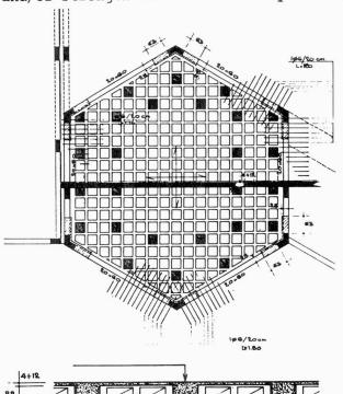
thickness having previously removed some of the tiles: small concrete blocks are thus created which act as keys improving the transmission of shear stresses (fig. 33). The extra thickness of the slab can be made variable with maximum at midspan, to save material and weight.
