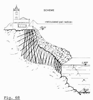
piles, forming a truss which makes a sort of reinforced earth crust, as a permanent stabilizator of the rock.
