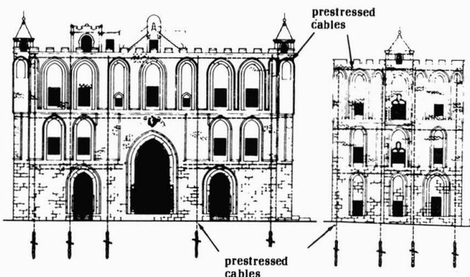
The walls are of sandwich type with outer tuffaceous blocks and poor filling material inside.
