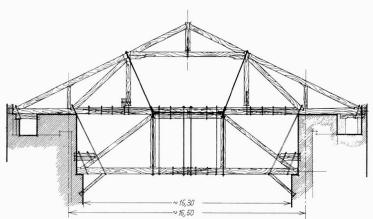
shown in fig. 3, relative to a truss forming the roof of a stage in a theater. The loads from the structures below are transferred to the selected joints by means of prestressed steel bars.
