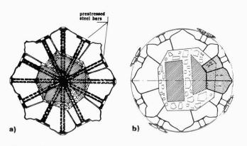
Improvements can be obtained by a-dopting prestressed diametral bars, whose effect is equivalent to that of a perimetral confinement.
