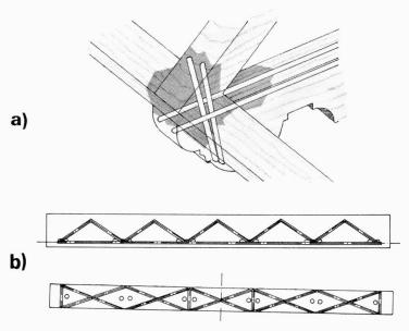
of wood can be removed and epoxy mortars cast in situ to reintegrate them. This is frequently the case of the extremities of floor girders or trusses encased into niches of the walls and subject to humidity: the intervention can consist of the reconstitution of the degraded parts with epoxy resins, possibly with the addition of fiberglass, as shown in fig. 4.
