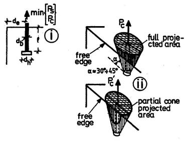
Fig. 45: i) Short anchors with anchorage head
