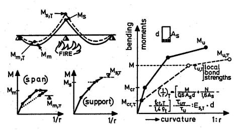
Fig. 53: A two span continuous beam after fire. An oversimplified model for the assessment of the redistribution of bending moments.
