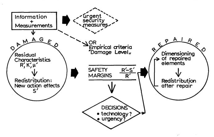
Fig. 1: A thinking model for redesign of buildings.R=strength, S = action-effect, K = stiffness,  $\mu$  = ductility
