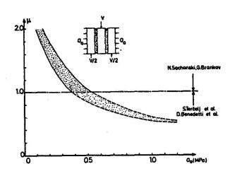
Fig. 7: Friction coefficients for masonry as a function of the average normal stress.
