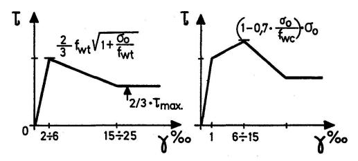
Fig. 41: Empirical data for shear deformation of brickwork infills
