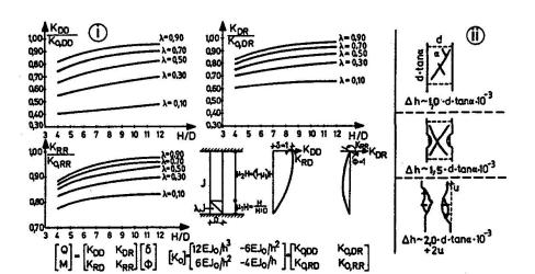
Fig. 50: i) Parametric calculation of stiffness indexes of a damaged R.C. column (Syrmakezis, Voyatzi, 1983) ii) Rough estimation of "settlement" of damaged columns
