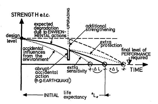
Fig. 55: The degree of ugrading, combined with the intensity of future environmental factors, may adversely influence life expectancy of buildings
