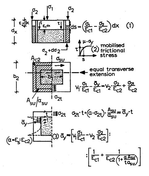
Fig. 39: Shearing and normal stresses developed at the "jacket/original column" interface
