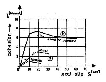
Fig. 5: Constitutive curves of adhesion (local stress-local slip)
