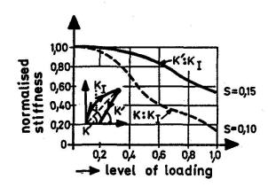
Fig. 31: Empirical values for residual stiffness after damage. A scattering equal to ±s should be taken into account
