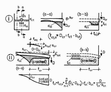
Fig. 11: A qualitative model for post-cracking displacement s due to dowel action
