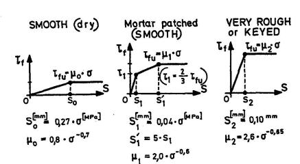
Fig. 6: Formalistic models for concrete-to-concrete friction, as a function of normal compressive stress "o" (MPa) and relative displacement "s" (mm)
