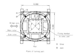
Fig. 2. Device to make constuction beam without any traffic disturbance
