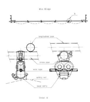
Fig. 1 Wire Bridge and Base Carry
