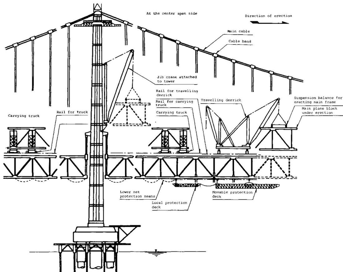
Fig. 9 Stiffening truss
