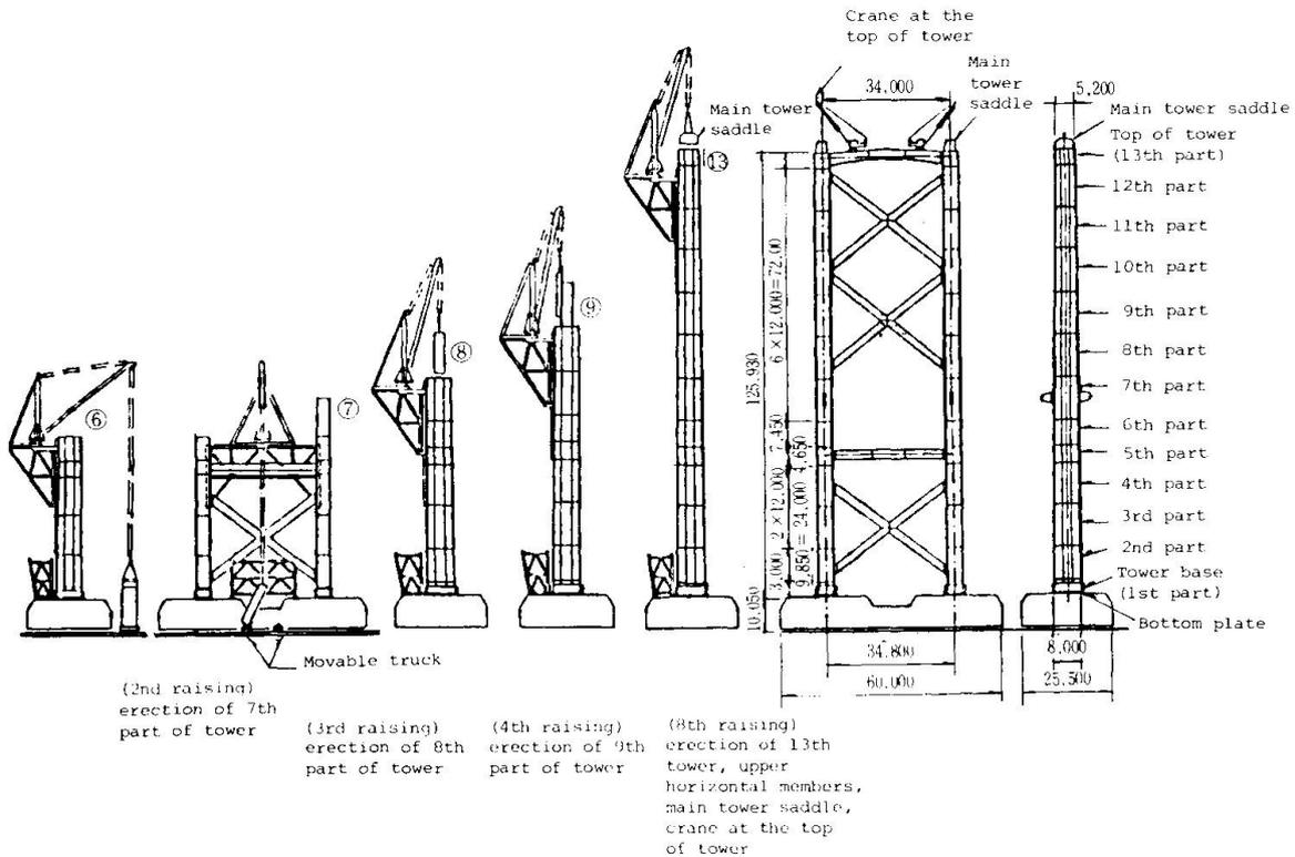
Fig. 6 Steps of erection of main tower
