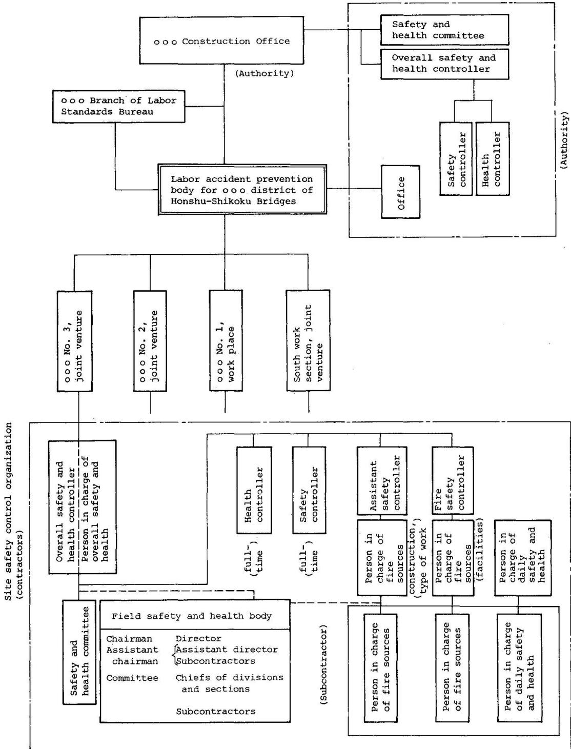
Fig. 2 An Example of safety control for the construction of the Honshu-Shikoku Bridges
