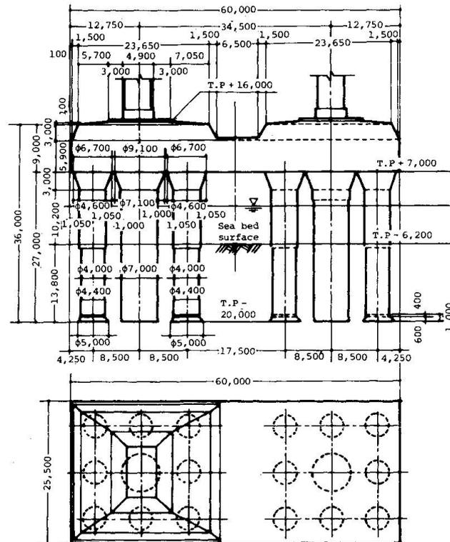
Fig. 3 Multi-column foundation
