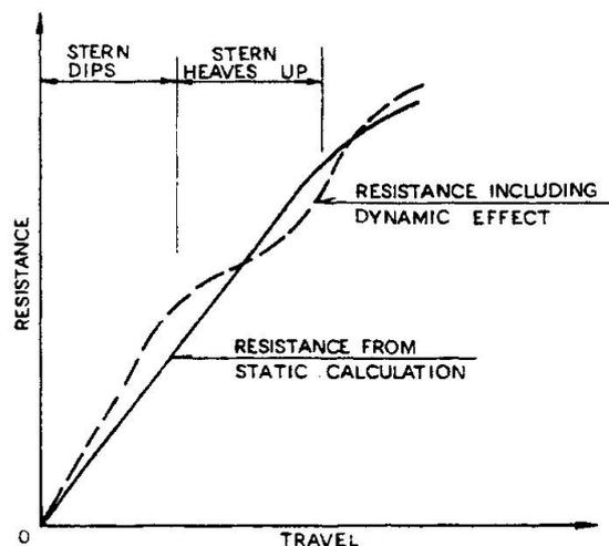
Probable shape of resistance curve, including dynamic effect, for vessel sliding up on a beach.
