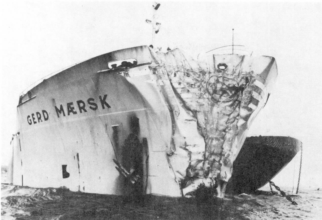
Fig. 2. Collision damage to tanker.
