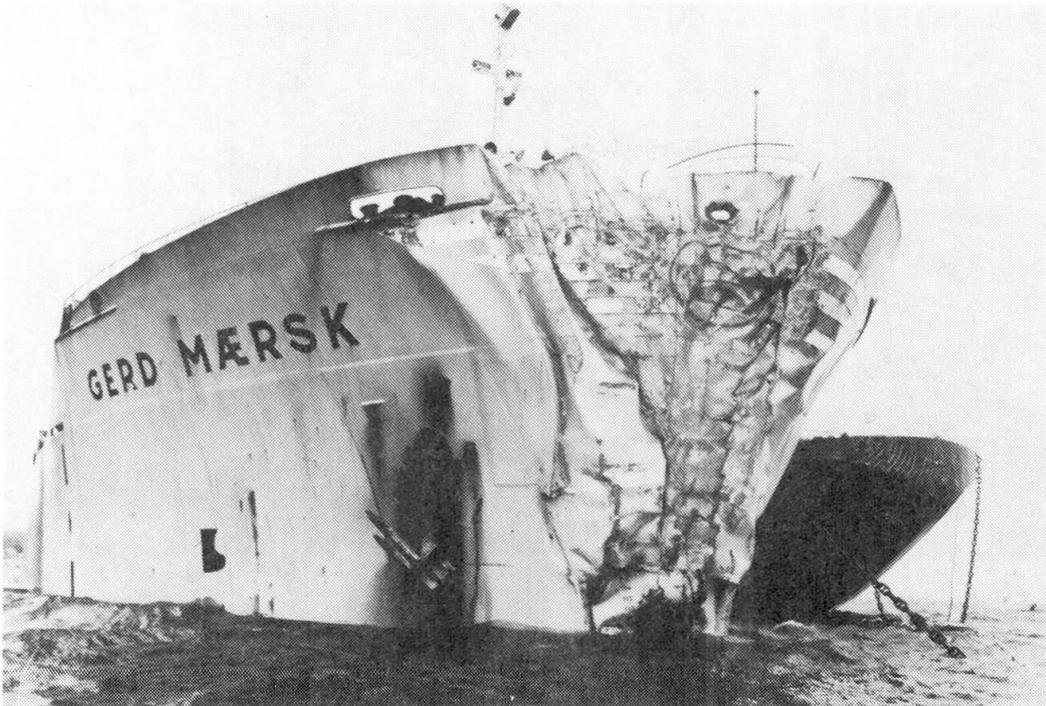
Fig. 2. Collision damage to tanker.
