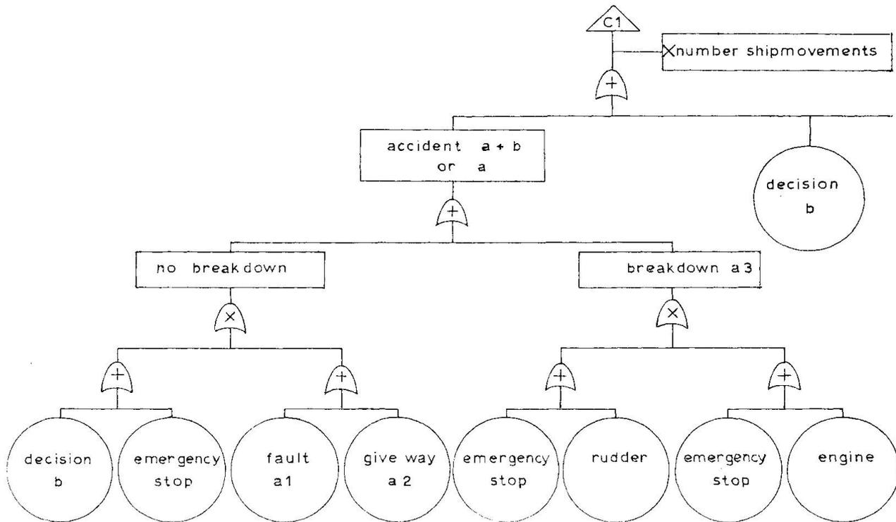
Fig. 6 Sub fault tree C1
