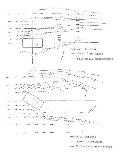
Fig. 3 Flow Pattern around the No. 5 Pier
