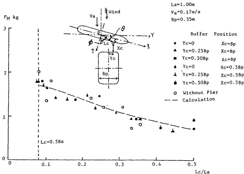
Fig.11 Impact Forces of Drifting Ship in Wind
