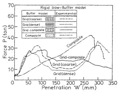
Fig.12 Comparisons between the Force-Bow Penetration Curves for Four Kinds of Buffer Devices
