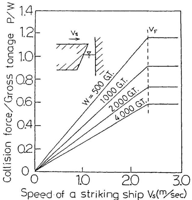
Fig. 10 Estimated Impact Forces at the Bow Collision
