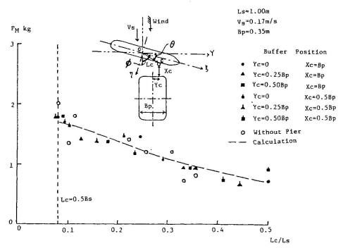
Fig.11 Impact Forces of Drifting Ship in Wind
