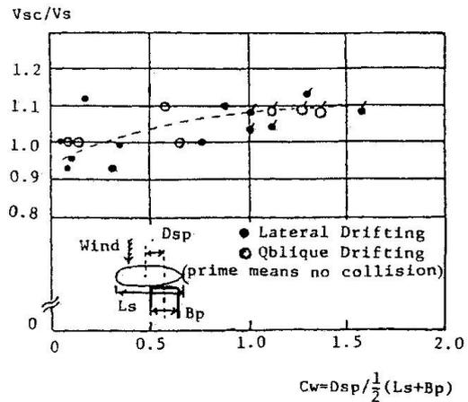
Fig. 9 Colliding Speed of Drifting Ships in Wind
