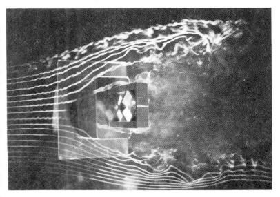
Fig. 4 Streamline around the Pier in Wind
