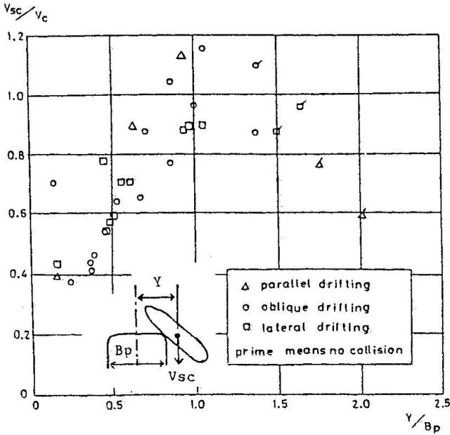
Fig. 8 Colliding Speed of Drifting Ships in Current
