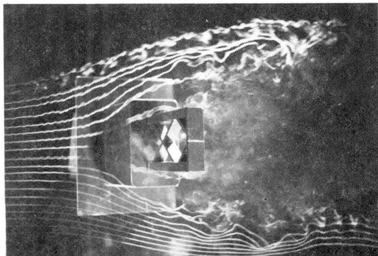
Fig.4 Streamline around the Pier in Wind
