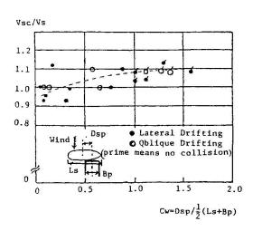
Fig.9 Colliding Speed of Drifting Ships in Wind
