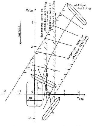
Fig. 7 Dangerous Zone to the Drifting Ship in Current
