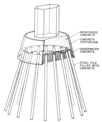
Fig. 9 Piled foundation of bridge pier
