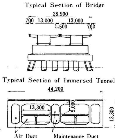
Typical Section of Immersed Tunnel
