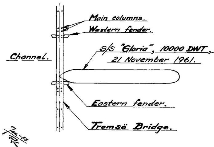
Fig. 3 Tromsø Bridge: Collision, November 1961. Dimensions of ship, channel and fenders.
