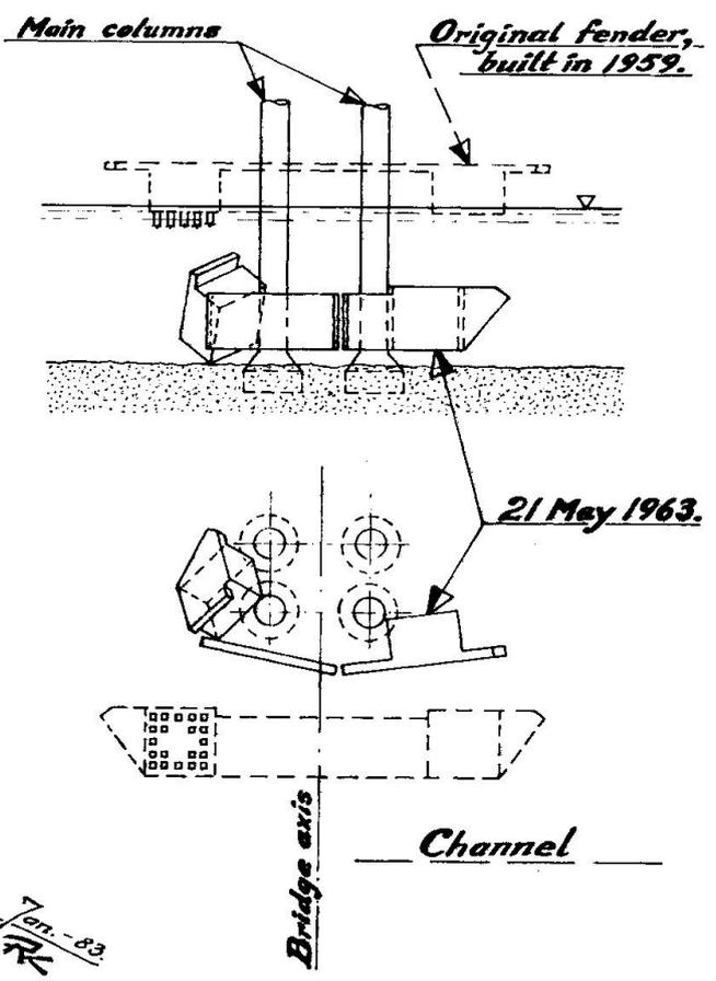
Fig. 4 Tromsø Bridge: Western fender before and after having been destroyed. (The destroyed fender was partly resting on heaps of broken piles, which are not shown on the figure).
