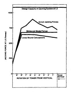
The actual values had a disturbing peak in them which was caused by a jammed shear lock. Without this occurence it is believed that the measured values would have paralleled the model values closely. Even with the jamming, the maximum jacking forces did not come close to the upper capacity provided in the recovery scheme.
