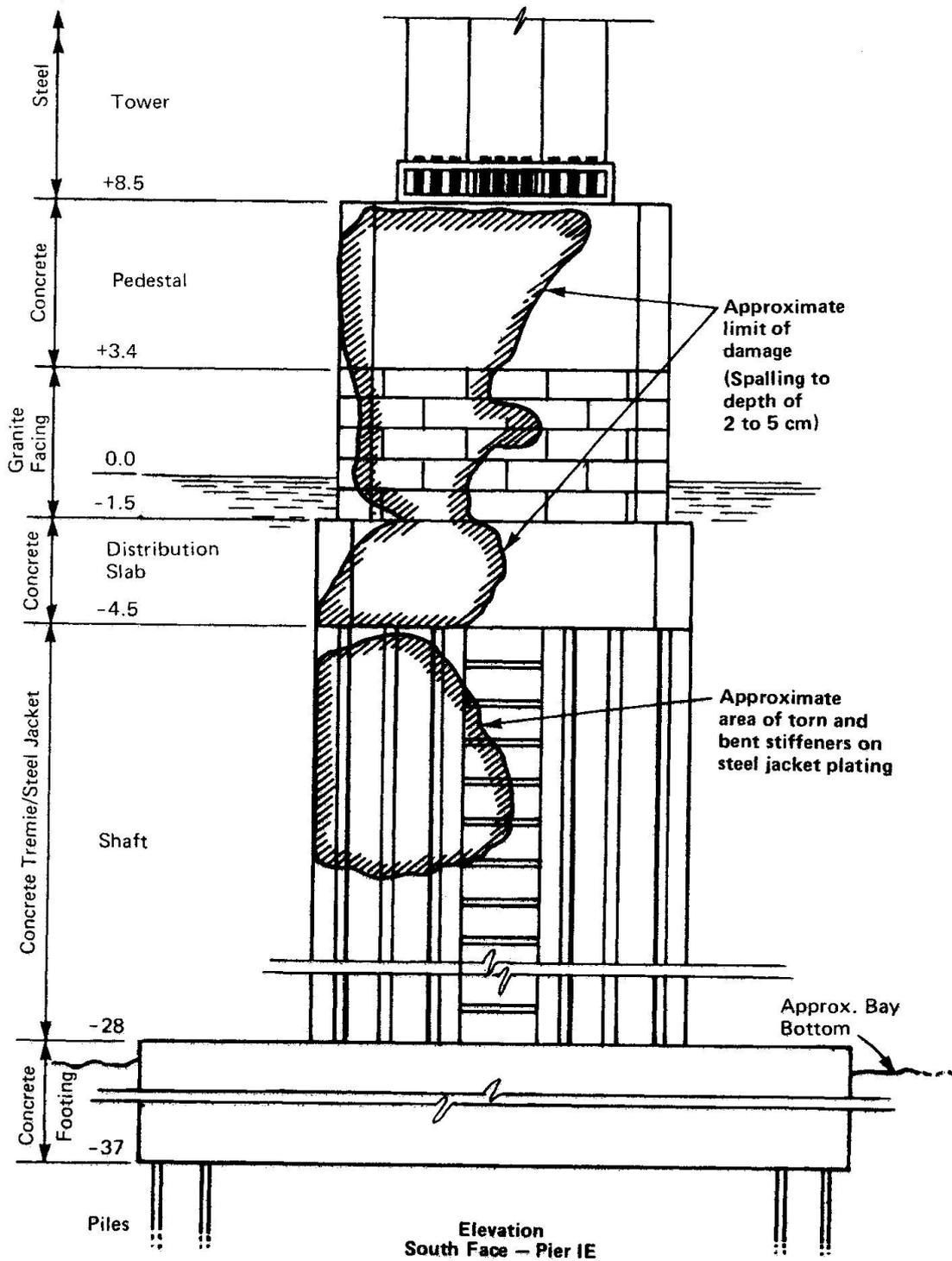
Fig. 4. Pier damage above and below waterline.
