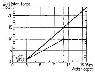
Fig 6. Design-forces due to shipcollisions for planned Oresundsbridge
