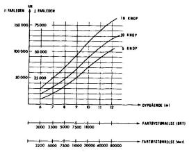
Fig 7. Shipcollision forces according to Nordic Recommendations
