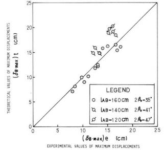
Fig.7. Comparison of the theoretical values of  $(\delta_B)_{max}$  versus the experimental ones
