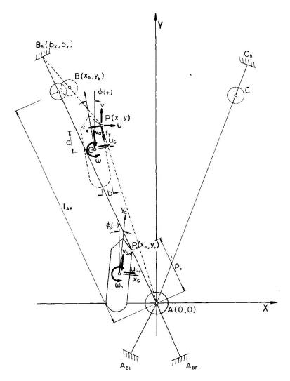
Fig.2 Co-ordinate system and symbol defenition of the collision-prevention device
