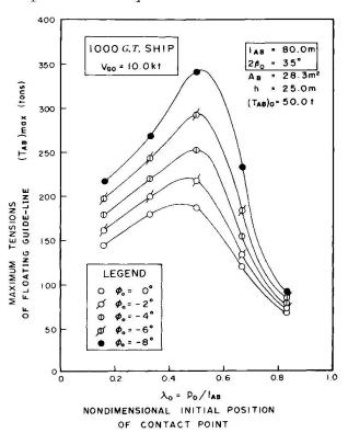
1000G.T. is approaching at a velocity of 10 knots;  $l_{AB}$  = 80 m;  $A_{B}$  = 28.3 m²;  $2\beta_{0}$  = 35° in which  $2\beta_{0}$  is the included angle between two guide-lines AB and AC; and  $(T_{AB})_{0}$  = 50 tf (490 kN) in which  $(T_{AB})_{0}$  is the initial tension of guide-line.
