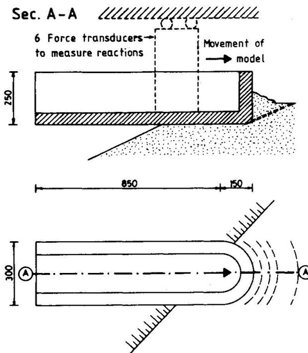
Fig.4 Principle for a test with the tanker model (dimensions in mm)
