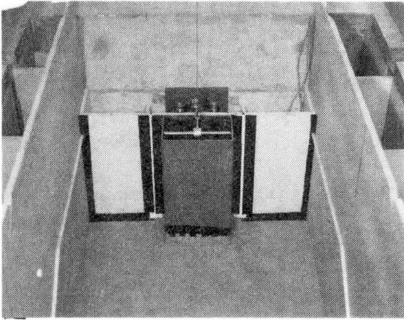
Fig.5 Pier model in the empty test pit
