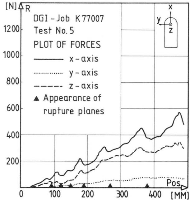
Fig.6 Components of forces plotted against the observed position (penetration) of the model
