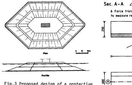
Fig.3 Proposed design of a protective island
