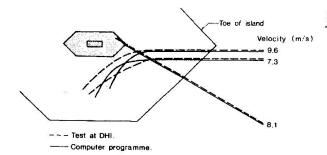
Fig.7 Examples of measured and calculated traces of a model tanker (from [1])
