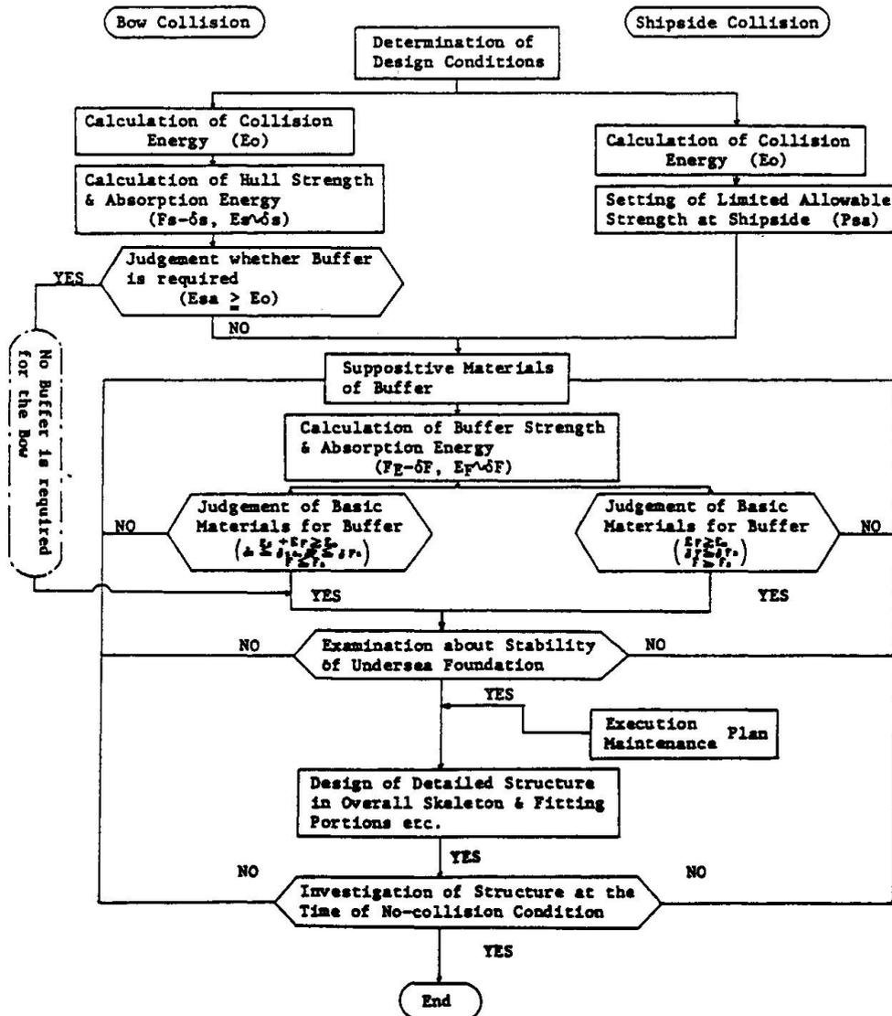
Fig. 8 Flow Chart for Design of Multi-cell Buffer
