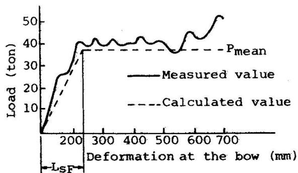
The crushed shapes and the maximum loads of the bow analyzed, have been checked with the results of statical crushing experiment by the models of 1/4 size of the 500 G.T ship and 1/8 size of the 4,000 G.T ship. Fig. 6 indicates the measured and calculated load-deformation curves of the experiment on the 1/4 model of the inclined bow of 500 G.T ship.
