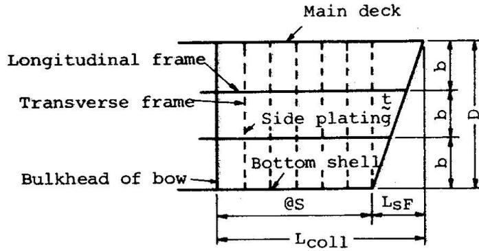
As a ship length  $L$  in common cases can conventionally be obtained depending on the ship size and a shape and dimension of the bow can be presumed using  $L$  as a parameter, the structure of the bow have been standardized as shown in Fig. 3 and Table-3, based on the investigation concerning to the actual navigation status in Seto-Inland sea.
