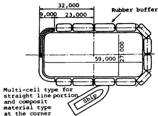
Fig. 7 indicates the general view of the buffer, and Table-4, -5, -6 indicate the ships under consideration, strength of the ship and the result of verification of the buffering function in collision.
