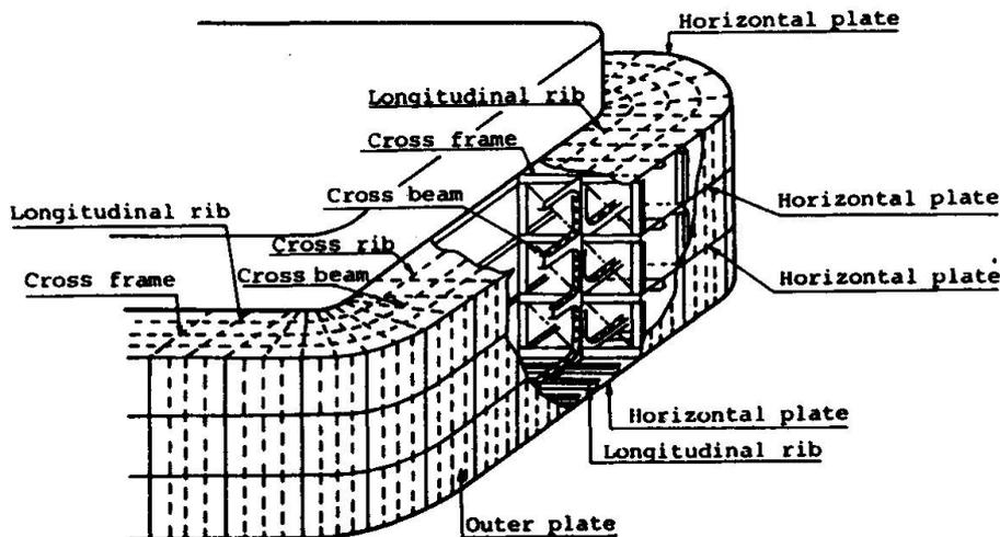
Fig. 2 Multi-cell Type Buffer
