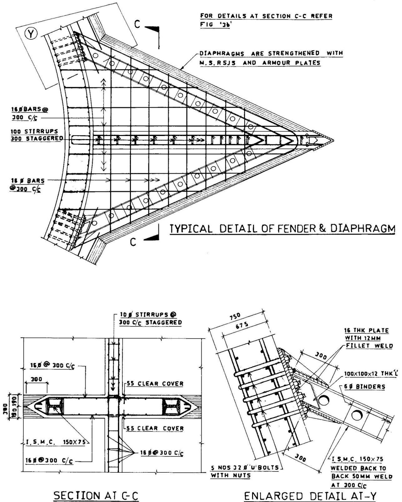
Fig. 3 Details of fenders for Zuari Bridge
