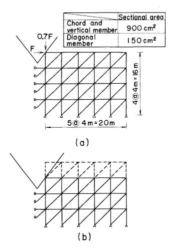
Fig. 9 Example of multi-layer truss
