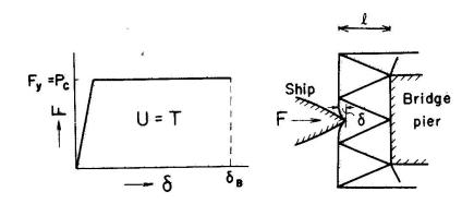
$\underline{\textbf{Fig. 1}} \quad \textbf{Load-deflection relation of buffer structure}$
