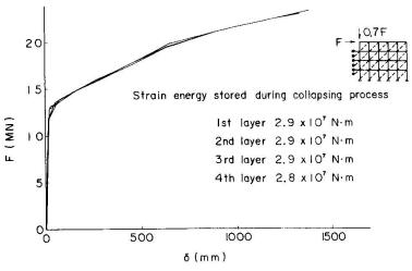
Fig. 10 Load-deflection diagram of multi-layer truss
