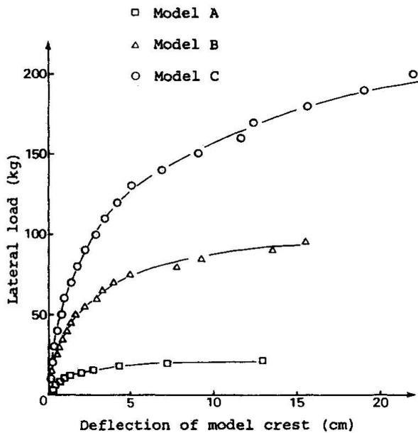
Fig. 7 Model crest deflection versus lateral load
