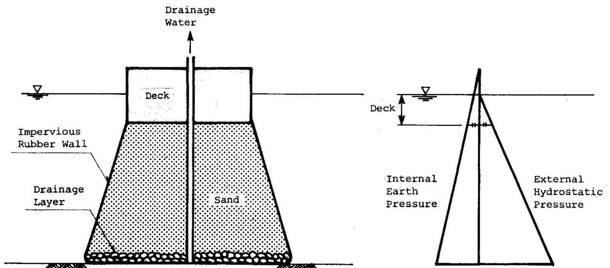
Fig. 1 Concept of Sandisle structures
