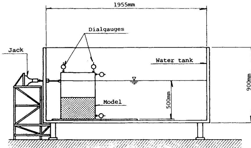
Fig. 6 Side view of test apparatus
