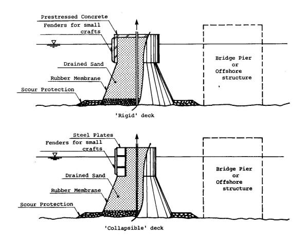
Fig. 5 Two types of ship collision barrier
