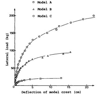
Fig. 7 Model crest deflection versus lateral load
