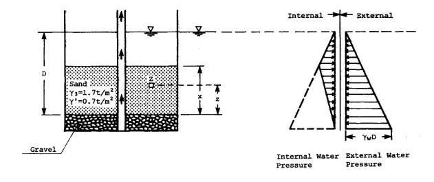
Fig. 2 Effective stresses in Sandisle construction
