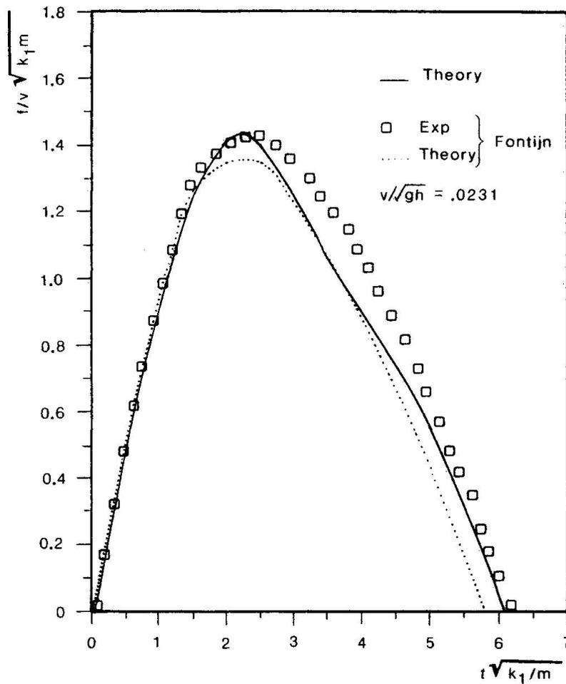
Fig. 2 Time History of Fender Force: Linear Fender
