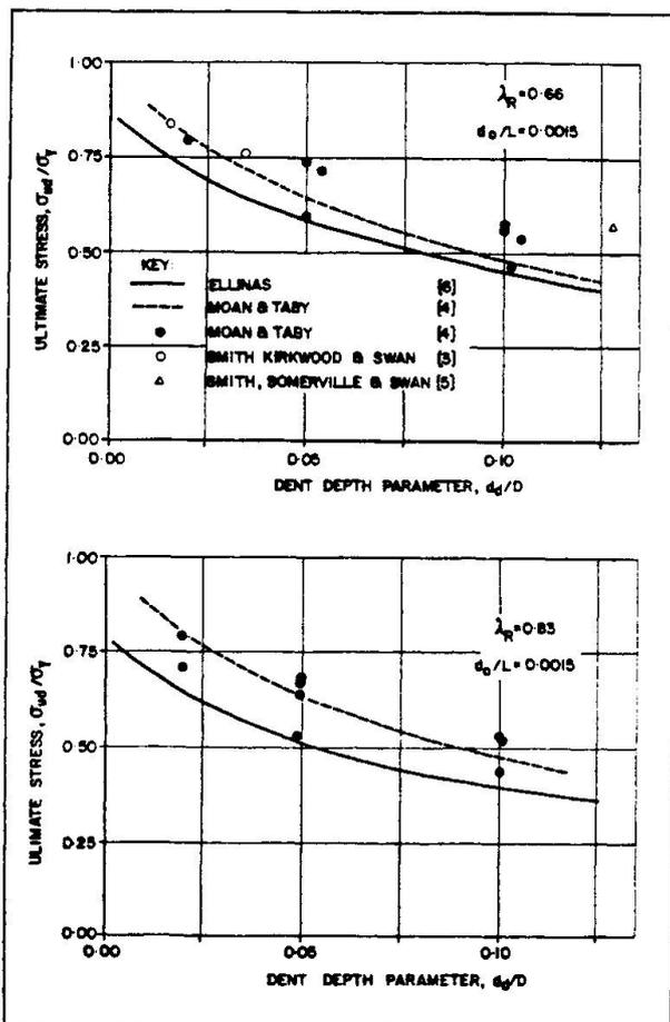
Fig.6 Comparisons for tubes with local denting damage only
