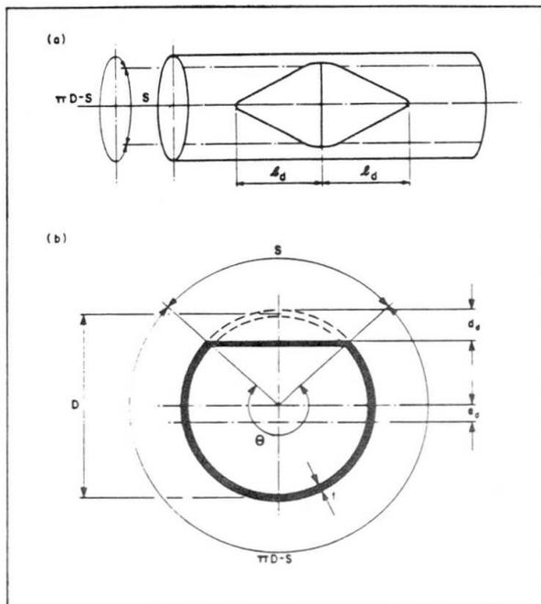
Fig.1 Dent geometry
