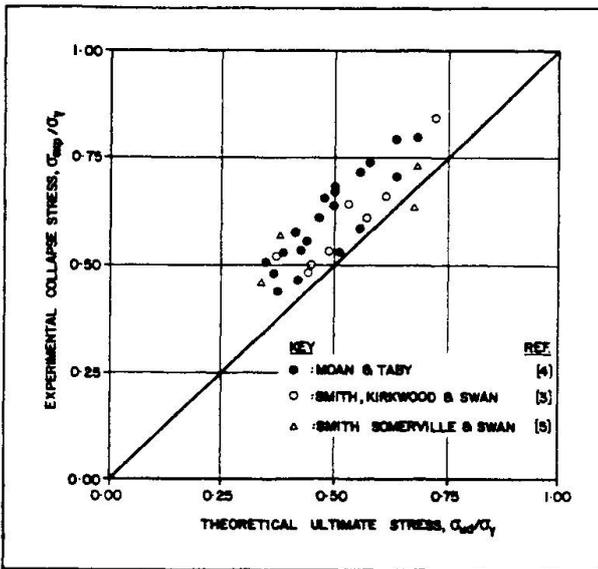
Fig.5 Theoretical and experimental comparisons for damaged tubes
