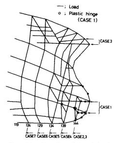
Fig.8 Idealized model of tanker
