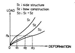
Fig.13 Load-deformation curve of bow and side structure
