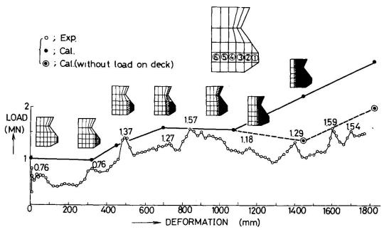
Fig.6 Load-deformation curve of tanker model
