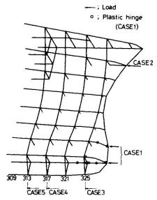
Fig. 7 Idealized model of container carrier
