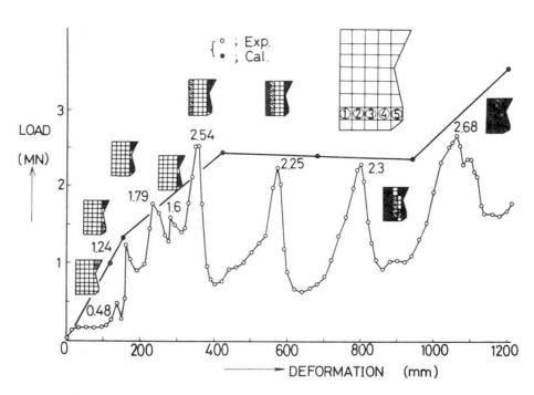
Fig.5 Load-deformation curve of container carrier model
