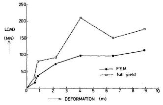
Fig.12 Load-deformation curve of ice strengthend ship
