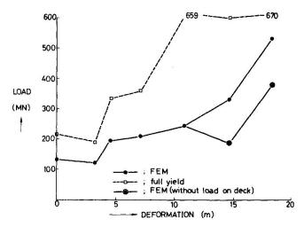
Fig.11 Load-deformation curve of tanker by FEM
