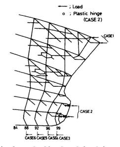
Fig.9 Idealized model of ice strengthend ship
