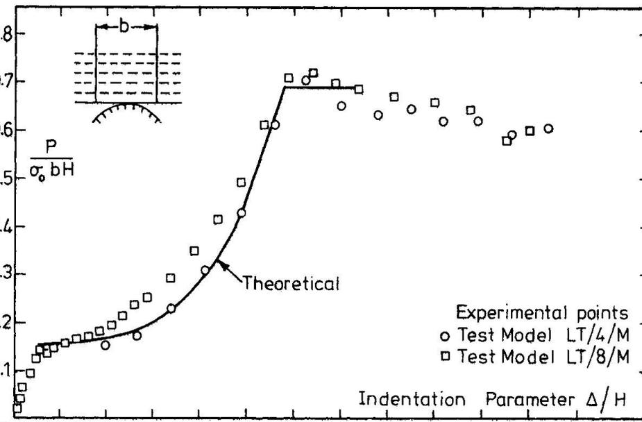
Fig. 3(b) Comparison of Experimental and Theoretical results: LT/4/M & LT/8/M
