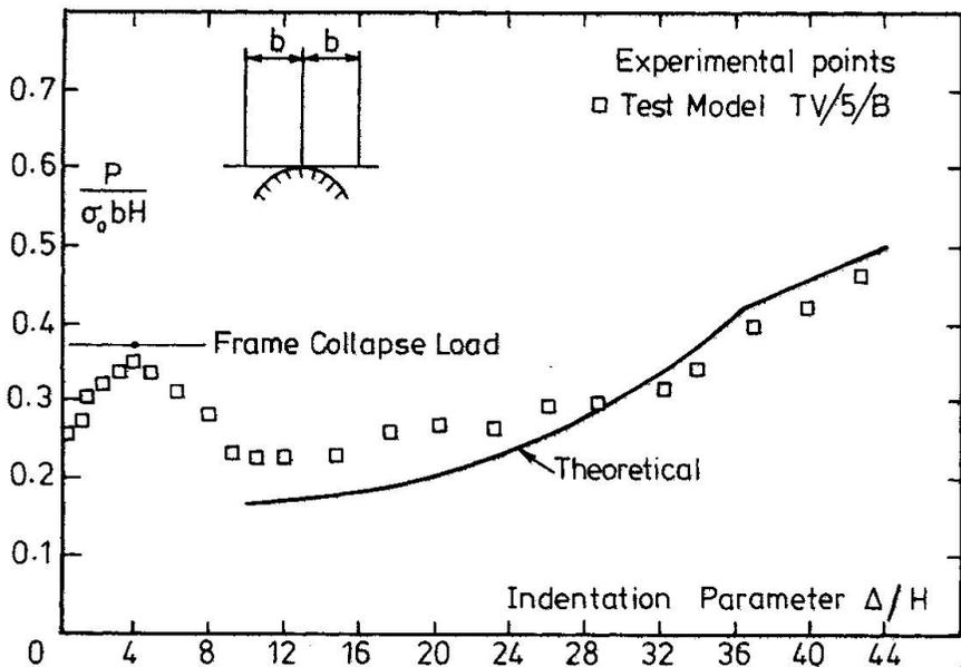
Fig. 3(c) Comparison of Experimental and Theoretical results: TV/5/B
