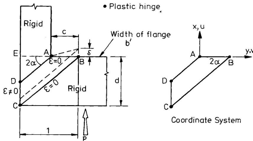
Fig. 5 Assumed Shear Collapse Mechanism
