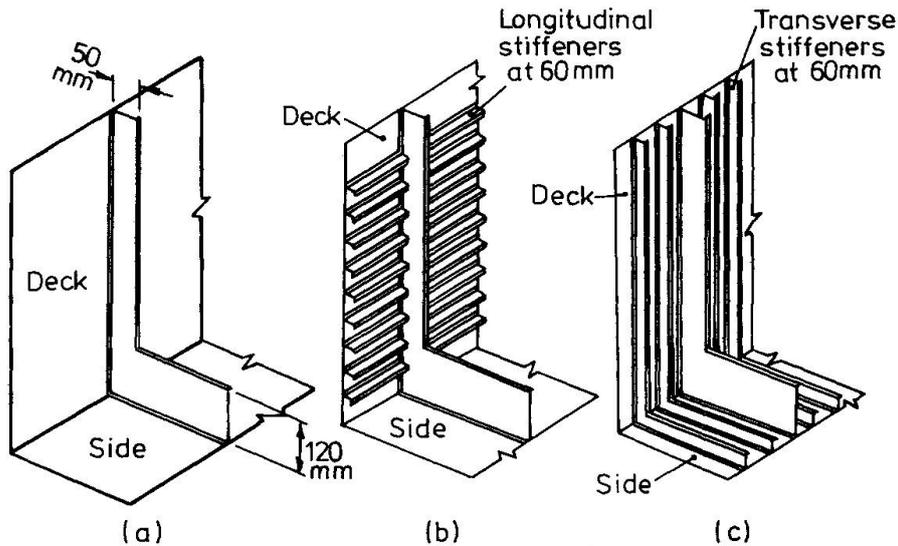
Fig. 2. Stiffener Arrangements used in Test Models
